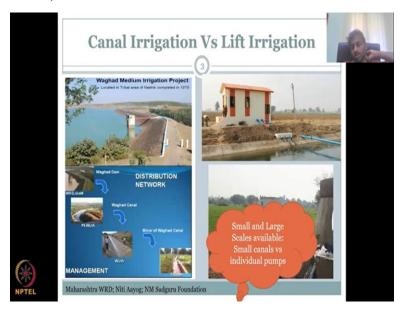
So, this is the very, very important difference between your canal irrigation versus lift irrigation. In your canal, you have water stored on a larger water spread area and from there multiple schemes are there to bring the water to the end farmer all through gravity. There is no pumps, it is only a gate and you open the gate or a small partition and then water flows.
