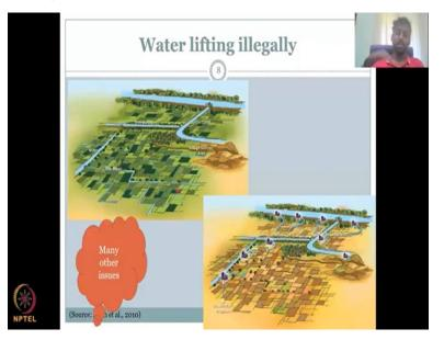
Let us go through this slide the last slide for today on how water lifting illegally is being done. So, for example this is the main river channel and there is or the canal from the big dam for irrigation and then there is a pump house which monitors the water pumps the water into the branch canal and from there it goes to the village service areas. Distribution this is a major distribution channel, minor distribution channel and then some more miners, so all these villages
