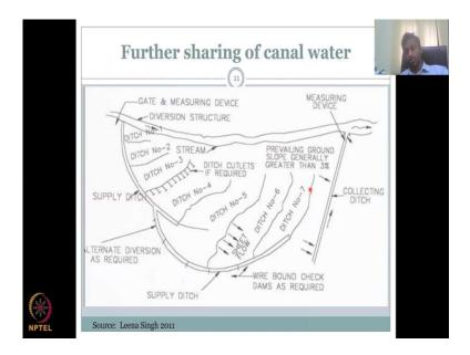
And it is done by like this. So, when the water is released, multiple ditches and smaller canals can be dug and taken out from the major canal which comes from the engineer structure of dam and that water can be intermittently supplied so that the groundwater recharge happens.
