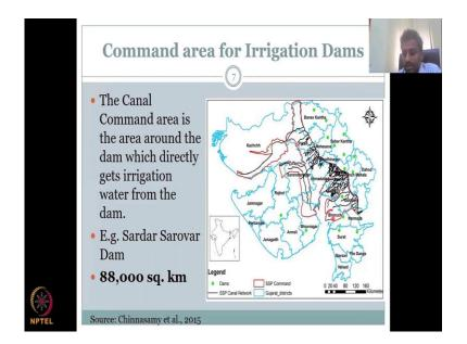
Because of this your crop area increases so I am just taking a case study of Gujarat from the previous slide that I have established a dam. So, the dam and the command area which is the red color while as the black is the canal network. So, you could see here that the water is stored and then release along the canals. Canal density might be high in some regions and low in other regions which is fine.
