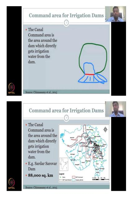
Let us discuss the command area as I said for irrigation dams. What is a command area? The canal command area is the area around the dam which directly gets irrigation water from the dam. So, for example, I will just double draw something for you to show first you have the dam each dam would have a area on the top and on the bottom. So, this is called the catchment area of the dam where all the rainfall, water pools together and comes to the dam and then you have a command area.
