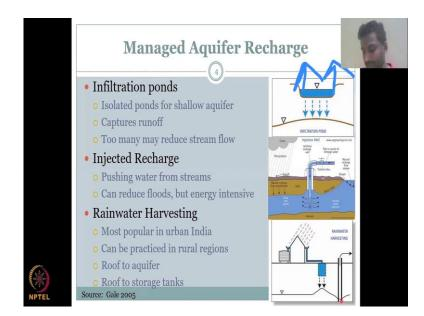
As I said, the infiltration pond which you see on the top, it is isolated ponds for shallow aquifers, it deals only with the shallow aquifer where on the bottom you do not do any change. You could just dig it up and then make sure that water is stored and it has space contact, contact with the ground and the ground slowly infiltrates the water to the aquifer.
