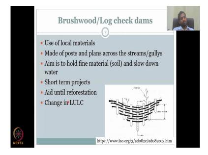
Use of local materials is how it is constructed, made of posts and plants across the stream, gully. So there are lot of posts which are wooden posts and then you have your plants and seedlings across the stream/gully. Aims to hold fine material soil and slow down the water. So because of the root zone, because of the soil plugs, it will actually prevent the sediments and slow down the water and more and more water would go.
