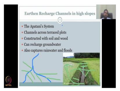
Then we have earthen recharge channels in high slopes. High slopes can have a small dam or a small check dam on the top and from there water is being sent to different locations. How are they sent? By channels, So the channels if it is coming as a concrete then it is not a nature-based solution, it is a constructed solution.
