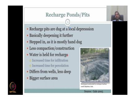
A recharge pit constructed for recharge of surface runoff in Rajasthan where the surface runoff is pooled into this recharge pit. And you can see that there is no concrete or no rocks and no cement etcetera. Everything is hand dug into the well and there was already depression there. So there was already a low-lying area. All they had to do is make it bigger, make it more into pooling water conditions and water would move slowly and then recharge.
