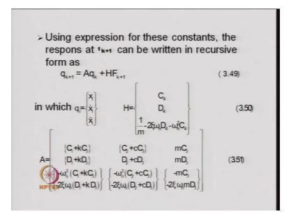
And that is what is done over here and once you are able to find out these quantities that is C 1, D 1, C 2, D 2, C 3 t D C, etcetera, you can write down the equation in this recursive form where u k plus 1 is equal a matrix a into q k plus h into F k plus 1 where q basically represents for all the 3 quantities in a vector form and a is a matrix consisting of these constants and the h is again a matrix consisting of some of the elements some of some of the constants of those equations.
