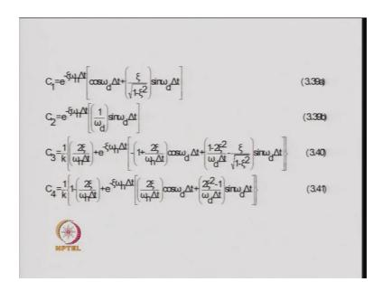
In these equations and you can see that these C 1, C 2, C 3, etcetera depend a delta t that is a time step and all other quantities are known that is omega d del omega d psi omega and etcetera.
