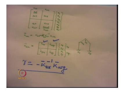
For example x 1, x 2, x 3, they are the rotations and these rotations are taken on the top. So, this is the 3 by 3 matrix corresponding to the rotational degrees of freedom and this is the matrix 3 by 4 that we are calling as ka K r u, this is the coupling between the rotational degree of freedom and the translational degree of freedom and this is these 4 by 4 is the translational degrees of freedom and the 4 by 4 square matrix correspond to that.
