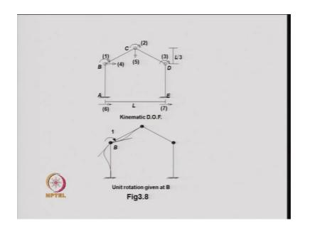
Next we take another example to illustrate the same r matrix; that means, how we can construct the r matrix for a pitched roof portal frame in this pitched roof portal frame, we have the 1, 2, 3; these 3 degrees of freedom are the rotational degrees of freedom and the 4 and 5; they are the translational degrees of freedom in addition to that we have 2
