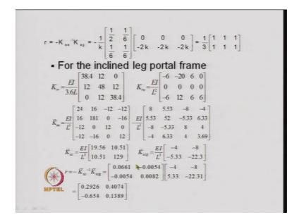
We calculated this quantity that is K s s inverse K s g and that turn out to be one third into 1 1 1 and 1 1 1. So, the 3 ground displacements share equal equally or share equally in producing the non support responses at the non support degrees of freedom.
