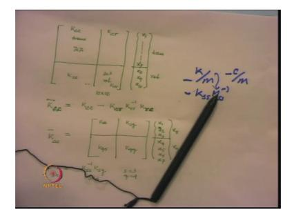
Which is a 10 by 10 matrix out of that the first 7 or 7 by 7 stiffness matrix corresponding to the 7 translational degrees of freedom they are grouped at the top and the 3 rotational degrees of freedom are grouped at the lower part of this vector, then we do this matrix con condensation using this relationship and condense the entire stiffness matrix to the translational degrees of freedom x 1 to x 7.
