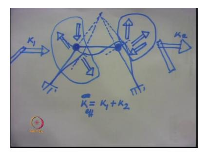
In order to obtain the stiffness corresponding to these degree of freedom let us try to recapitulate how we can find out the stiffness of the system we are interested in obtaining the force required to produce unit horizontal displacement over here.
