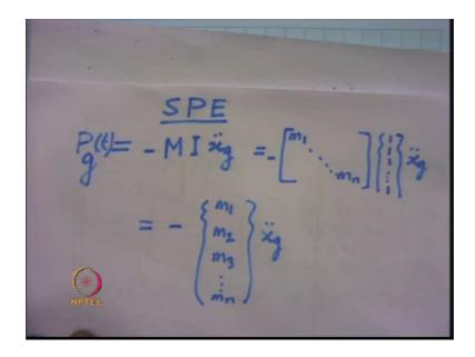
And this is discussed over here say if it is a single point excitation system then minus M I x double dot g that is the right hand side force vector and if we expand it this is a diagonal mass matrix I is a vector for the multi storey buildings 1111 into x double dot g that gives a right hand side load vector as minus m1, m2, m3 up to m n into X double dot g.
