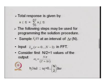
The summary of the frequency domain analysis is the given over here that is sample X double dot g t at an interval of delta t that will give a value a N values of the ordinates, then input these sample values in FFT then consider the first N by 2 plus 1 values of the output and we get the Nyquist frequency and the Nyquist frequency is given by this and we obtain h j i omega which is the complex frequency response function for the single
