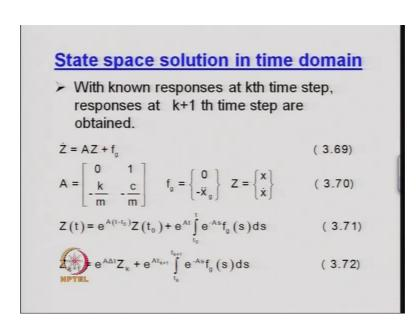
One is the Duhamel Integral. Other is the New Marks beta method. Both the integrations schemes were cast in the recursive form so that if one knows the displacement, velocity, and acceleration at k-th time, then one can find out the displacement velocity and acceleration at k plus one-th time. Provided the force acting at the k plus one-th time is known, in fact in all cases the load is specified or load is known before hand therefore there is no problem.
