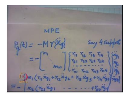
If we consider the multi support excitation then the this is the form of the equation that is minus m into r into x double dot g this is the mass matrix diagonal mass matrix the r matrix say we are considering 4 support excitation then it will be a n multiplied by 4 matrix, n is the number of degrees of freedom and the r matrix would look like this and x double dot g1 and x double dot g2 and x double g3 and x double dot g4 they are the support excitation.
