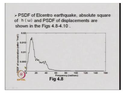
So, multiplying them together we get the value of the power spectral density function of the response here in this figure the power spectral density function of the elcentro ground motion taken from the appendix that is plotted.
