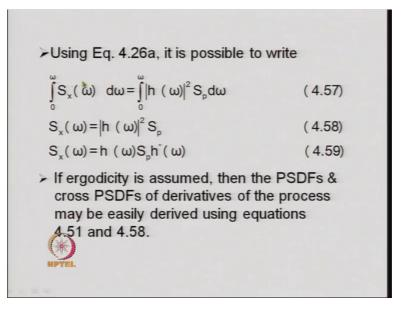
Now if we look into this 2 integrations then from that it immediately follows that S x omega becomes is equal to h omega absolute square into S p and S x omega also can be written as h omega into S p multiplied by the complex conjugate of h omega because this complex conjugate of h omega and this h omega they becomes equal to absolute value square.
