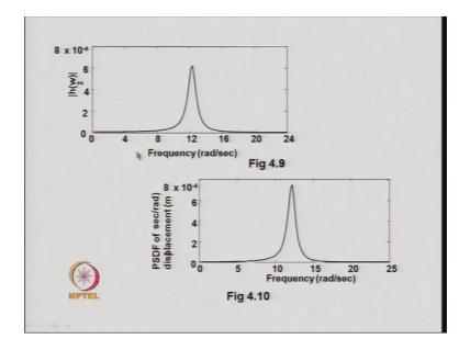
In this equation the frequency response square h omega absolute square that is plotted against frequency and the multiplication of these 2 gives you the power spectral density function of the response and that is again plotted over here against frequency.
