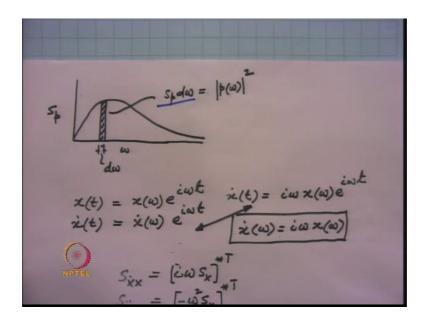
Then that d omega into S p; S p that becomes equal to absolute value square at this particular omega and if we sum up all the absolute value square in this diagram then they would be equal to that sum will be equal to the means square value of the process that we have seen.
