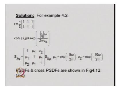
I(n which we had a 3 supports and two nonsupport degrees of freedom u 1 and u 2 and we discussed how we obtain the cross power spectral density function terms of the power spectral density function matrix of the excitation.
