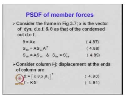
Next you come to the power spectral density function of the member forces, once we obtain the power spectral density function of the displacement that is the displacement of the various translational degrees of freedom, then from that one has to obtain the power spectral density functions of the member end forces and for that we take say this particular frame and here.
