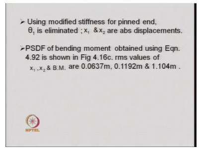
And the displacements and bend r m s values of the displacement and bending moments where obtained for different quantities.
