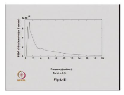
Degree of freedom 5 and one can see that the for degree of freedom 4 the value is more compare to the value of the power spectral density function of the degree of freedom 5, because this is of the order of ten to the power minus 5 the other one is of the order of 10 to the power minus 3. And the area under the curve of course, provides us the root mean square value of the absolute displacement of the degree of freedom 4 and degree of freedom 5.
