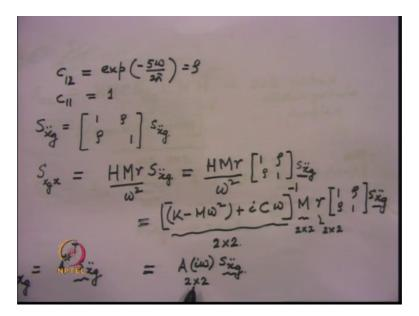
That is the relationship that we have used and once we take that relationship then what first we have to obtain is the cross power spectral density function matrix of excitation S x double dot g is the elcentro power spectral density function, and the C11 C 22 C 12 terms they will be this will be 1 1; obviously, and this will be the row a row will be equal to exponential of minus 5 omega by 2 pi is equal to row.
