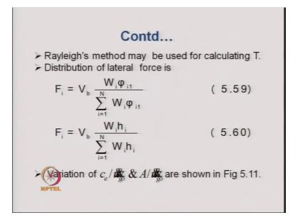
The Rayleigh's method is used for calculating the time period T. Note that many of the codes apart from prescribing the Rayleigh's method for calculating the time period T, they also provide some other empirical equations for calculating the time period T. Distribution of the lateral force follow the same pattern as the National Building Code of Canada that is h i having a power of unity that is k is equal to 1.
