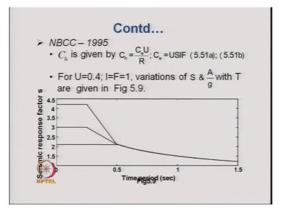
Next comes the National Building Code of Canada 1995. Here the seismic coefficient C h value is given by C e into U divided by R, where R is the reduction factor. In the previous case we have not talked about the reduction factor. Here also although R is there; that means, the seismic forces which are calculated by the formula is reduced by a reduction factor that the same thing is done in the case of IBC, but we have not shown
