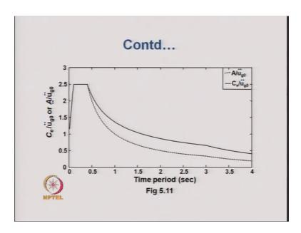
This is the comparison of the C e, the seismic coefficient value, normalized with the ground acceleration and the spectral acceleration normalized with the ground acceleration and one can see that the spectral acceleration is generally lower than the seismic coefficient in the higher time period range.
