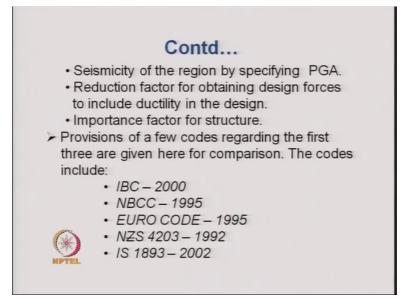
The next important thing that is specified by the code is the seismicity of the region by specifying peak ground accelerations.
