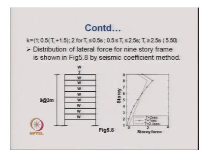
For example in this particular case that is uniform the International Building Code the 3 values of k are recommended, that is one, then next is 0.5 into T 1 plus 1.5 and the next one is 2 they are valid the first one is valid for time period less than 0.5 second that is k is taken as unity for time period less than 0.5 second. For time periods between 0.5 seconds to 2.5 second the value is taken as 0.5 into T 1 plus 1.5 and when T 1 is greater than 2.5 second, then the value of k is taken as 2.
