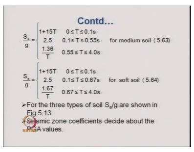
For the medium soil these values are little bit changed. The central portion that is of the curve that remains constant that is 2.5 and the initial phase that also remains same, that is 1 plus 1.5T. Only the last segment of the curve that changes it is 1 by T for hard soil. For medium soil it is 1.36 by T and for soft soil it is 1.67 by T.
