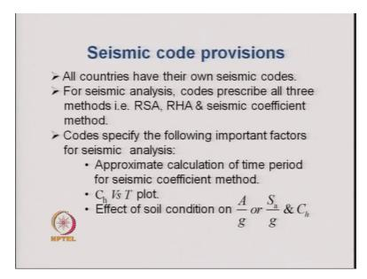
Here, we are not going to discuss all issues, we will be discussing only about the first 3; that is, the approximate calculation of time period for seismic coefficient method, then we look into C h versus time period plot and the effect of soil condition on A by g or S a by g and C h with T. So, our discussion here would be mainly centered around these 3 things which are given in the code.
