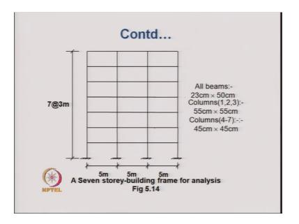
The all beams they have a dimension of 23 centimeter by 50 centimeter. Columns from 1, 2, 3, first 3 floors we have 55 centimeter by 55 centimeter column size and for the upper floors the column size are 45 centimeter by 45 centimeter.
