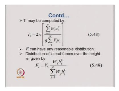
Next, the time period maybe computed by an equation 5.48 and this is given for the seismic coefficient method. If you are using the seismic coefficient method for finding out the seismic forces induced in different members of the structures, obtained by seismic coefficient method of analysis, then the time period that is calculated is by this formula.
