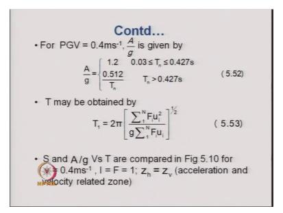
For the peak ground velocity of 0.4 meter per second the A by g or the spectral acceleration normalized with g is given by this equation that is equation 5.52 it is equal to 1.2 for a time period which is less than 0.427 and greater than 0.03 that is for the initial portion of the time period and for larger time period that is time period greater than 0.427 the S a by g is given as 0.512 by T n. Again, here we can see that it is inversely proportional to the time period.
