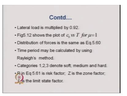
The other features of this code, is a lateral load is multiplied by a factor of 0.92. Then figure in the subsequent figure 5.12 we will show the plot of c b versus T for mu is equal to 1. Distribution of forces is the same as equation 5.60, that is, the same distribution W i h i divided by W i h i summation over all the storeys. Then the time period may be
