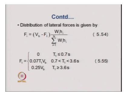
So for as, the distribution of the lateral force is concerned, the equation that is used is somewhat different than the International Building Code. In the International Building Code we had W i H i to the power k and the value of k could be 1, could be 2 and could be in between 1 and 2, but here it is the value of k is simply is equal to 1, that is why it is W i H i divided by sum of W i H i over all the force.
