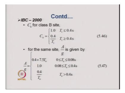
First, let us take the International Building Code. The seismic coefficient C h for class B site is given by equation 5.46. The class B site specifies certain zone in which peak ground acceleration is specified and for that the C h values are shown by this equation.
