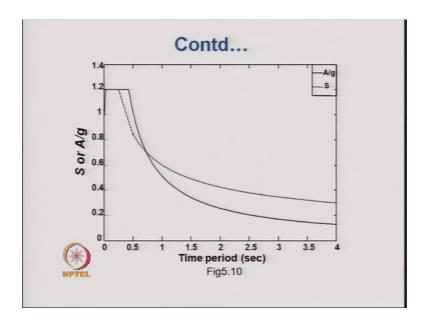
For that the curve is shown over here and one can see that the S curve that basically gives a higher value than S a by g.
