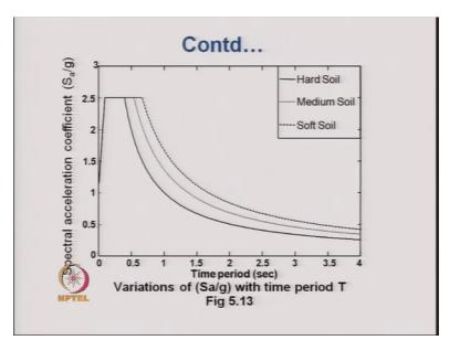
For the 3 types of the soil the S a by g are shown over here and one can see that for soft soil and for greater time period the S a by g coefficient is more. That is, for the soft soil we expect more amplification to take place.
