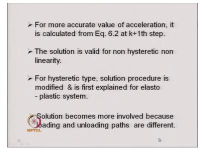
Now this kind of solution is valid for non hysteretic non-linearity, but if you are going to utilize these type of incremental solution for hysteretic non-linearity or hysteretic type of non-linearity then the solution procedure is modified and it will be explained with the help of the most simple type of idealization of the hysteretic type of non-linearity that is elastoplastic system.
