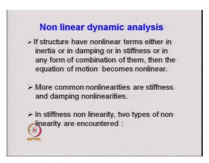
Now, what we mean by the non-linear dynamic analysis over here is that if the structure have non-linear terms either in inertia or in damping or in stiffness or in any form of combination of them, then equation of motion becomes non-linear; however, the more common nonlinearities that arise are due to the stiffness nonlinearity and the damping nonlinearity the inertia nonlinearity is hardly encounter. So, here we will be mostly talking about the nonlinearities arising due to the stiffness.
