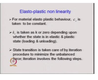
Therefore, what we do we constantly track the responses of the system at every time step, when we use the elastoplastic non-linearity and we use the same incremental solution then we only concentrate in the material non-linearity and we assume that the damping remains constant that is C t is constant at all times.
