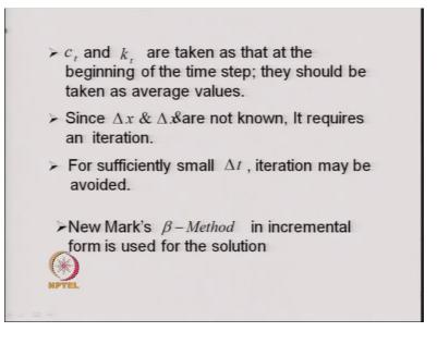
If we go for the analysis in which we do not have the hysteretic type of nonlinearity that is we have the general or geometric nonlinearity that we had shown before in this curve then we can see that during the interval delta x or during this interval of time delta t the stiffness changes from this value or the from this value to this value.
