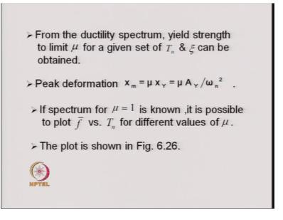
From the ductility spectrum yield strength to limit mu for a given set of T n, T n and psi can be obtained.
