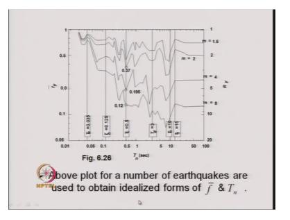
So, that we can see over here in this particular curve the f bar y and T n that is plotted over here for different values of the mu. So, there mu is equal to 1.5, mu is equal to 2, this is not m. So, there will be or all mu equal to 1.5 or 2, 4, 6, 10 so on and for these we have curves plotted these curves are nothing, but f bar y against a T n and that is the aim that we had.
