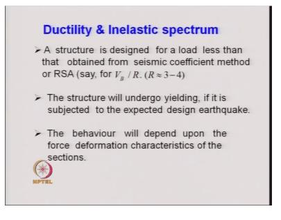
After that we discussed a very important topic called the pushover analysis in earthquake engineering. The pushover analysis is a is a very good equivalent static non-linear analysis of structures for earthquake with the help of pushover analysis we try to understand the elastic behaviour of the structure after the yielding during the earthquake, and also try to see the performance levels of the structure at different at stages of the earthquake loading.
