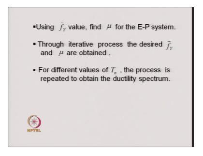
Then what we do that that interpolated value of f bar y and the mu this interpolated value of f bar y now is used in the equation 6.38 and it is solved, and value of mu is obtained and if you find that the value of mu that we have interpolated and the value of mu that we have obtaining from equation 6.38, if they are same then we say that a convergence is taken place otherwise what we do we through iterative process we find out the values of f bar y and mu.
