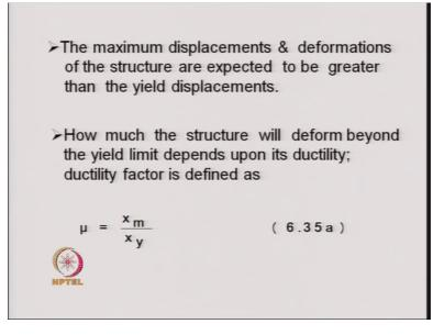
The maximum displacements and deformations of the structure are expected to be greater than the yield displacements, and that is that gives rise to the concept of ductility.
