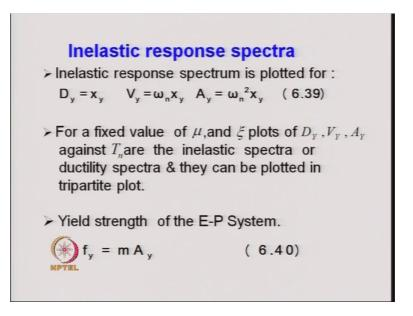
Next, we come to with this understanding of the ductility, we come to the inelastic response spectrum or the definition of the inelastic response spectrum and how one can construct the inelastic response spectrum.
