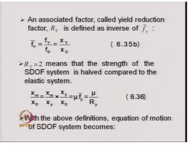
So, it from these equation one can say that provided we know x n f bar y at x 0 one can calculate the value of a mu, that is one of the equation merging out of that equal six point or relationship we merging out of equation 6.36 is that, x my by x 0 is equal to mu divided by R y and R y is a reduction factor it is nothing, but inverse of f bar y.
