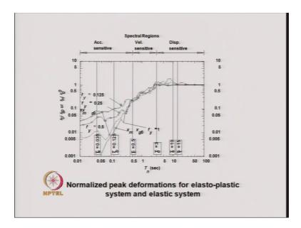
We on this figure we can see that we have the on this ordinate we are plotting x dot 0 divided by psi 0 and divided by x 0 divided by x g 0 and this is x m divided by x g 0.
