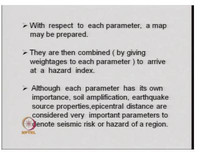
With respect to each parameter a map may be prepared. They are then combined by giving weightages to each parameter to arrive at a hazard index.
