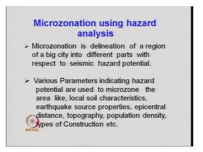
So, that is what is done in a microzonation. So, now, let us try to formally define the microzonation. Microzonation is delineation of a region of a big city in to different parts with respect to seismic hazard potential.
