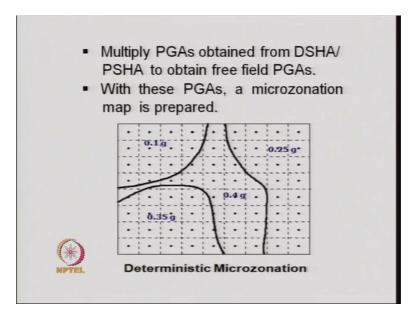
And multiply the PGAs that we have obtained and from the DSHA or PSHA analysis by the amplification factor and accordingly can prepare a microzonation map.
