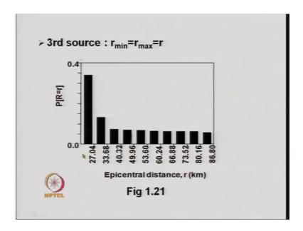
So, here for example, for the first source the probability of occurrence of earthquake with epicentral distance of 27.04 is about 0.336.
