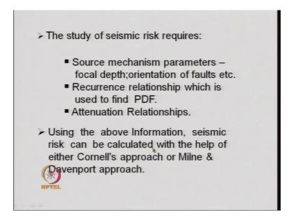
The study of seismic risk requires source mechanism parameters that is the focal depth orientation of fault etcetera, recurrence relationship which is used to find out the probability density function of the magnitude of earthquake that is what we have seen before and the attenuation relationships again we have used this attenuation relationship in connection with PSHA.
