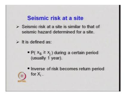
So, therefore, given the seismic hazard curve 1 one can find out the probability of occurrence of just 1 event and exceedance of at least 1 event and given the probability of exceedance for or the earthquake for a given period one can find out what is the average rate of exceedance the value of lambda that we have calculated in the second problem.
