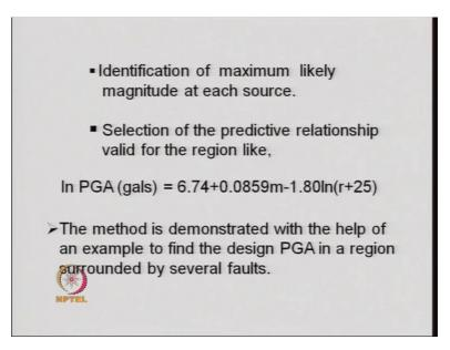
As I told you these attenuation relationship provides you the average value of the PGA and to this equation a standard deviation is specified because it is assumed that the peak ground acceleration and for a given magnitude of earth quake varies log normally.
