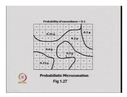
This one shows the probabilistic microzonation. Here the numbers over here associated with each sub region shows the probability of exceedance of 0.25 level of peak ground acceleration is 10 percent. So, we take 10 percent probability of exceedance that is 10 percent risk and based on that one can design the buildings with this peak ground acceleration.
