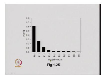
So, probability of occurrence of that magnitude of earthquake can be obtained for source 1, source 2 and source 3.
