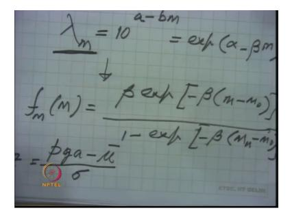
Any peak ground acceleration PGA minus is average value divided by its standard deviation this is the quantity z. Now, one can find out this normalized quantity and since it is assumed that the peak ground acceleration log normally varies, therefore this normalized quantity also varies log normally.
