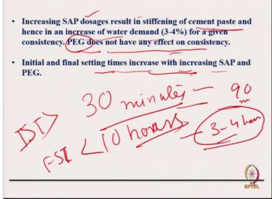
So increasing SAP dosages result in stiffening of cement paste and hence in an increase of water demand. Sometimes some of those SAP that is super absorbing polymer absorbs too much of water, so that will disturb the setting process, stiffens it quickly. So cement paste hence initial water demand might increase for a given consistency. Polyethylene glycol does not have any effect of this one, initial and final setting time increase with increasing SAP and
