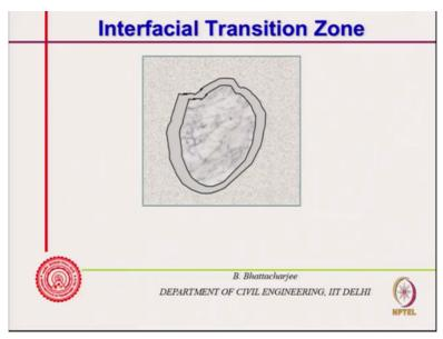
So this is the aggregate mortar interface, this is the aggregate mortar interface right, and that is ITZ.
