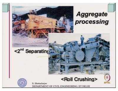
So if you have to remove there are separating screen, there are Magnetic Roll Crushing all these are there. Right, separating and roll crushing separating through screen and fine ones are separated out roll crushing. So this is process actually.
