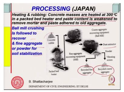
Heat it and rub, so concrete masses are heated to 300 degree centigrade in a packed bed heater and paste content is weakened to remove mortar and paste adhered to old aggregate. So this is a processing part other than getting, collecting, crushing, getting into the right sizes, now this is something more.
