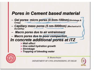
So pores in the cement base systems in fact in geopolymers also you will have pores. Although you are no using opposite link. Every all of these inorganic system because whenever you are adding water to react and solidify, all the water you know if it is consume and space fill by water if it is fill by that solid product then you will have no porosity. But usually that will not happen.
