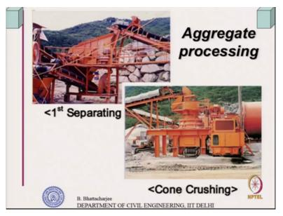
So, then separating using screens larger size to finer size. There can be Cone Crushing after that, so there are several stages of the crushing of this demolition waste in the mean time you have to remove the metals and other product right.
