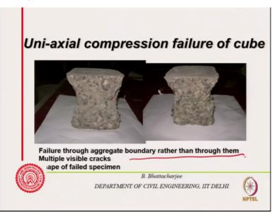
Now therefore, we should see how the aggregates you know role of aggregates and how we can reduce it all? Now this is what I show you or telling you sometime related to strength, you will find that failure always occurs with the normal strength concrete. Failures always occur at the aggregate mortar interface. You know aggregate mortar interface.
