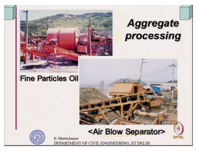
And then find particle or oil separation finer particle because you know decantation rate of the particle going through the material through liquid Stocks Law differs. So through oil you can do some separation. Air blow separation for very fine particle.
