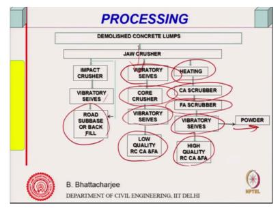
All right, so demolish concrete lumps I think I will stop after processing. Demolish concrete lumps that is why it comes goes to a jaw crusher and then from the jaw crusher it can go to impact crusher, vibratory sieves, this you can use in road subbase or back fill.
