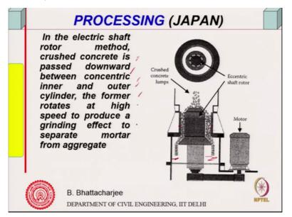
Okay, in that there is another kind of electric rotor shaft method, this is another one same you know process. This is passed downward now crushed concrete lumps are passed downwards, there is a of course a motor which it cause things to rotate and it is passed and this is one side of it Eccentric shaft is there, there is an Eccentric shaft and this rotates and this crushes against the wall, crushes against the wall.
