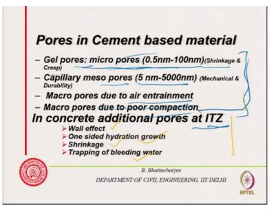
So therefore this ITZ, you know ITZ is a other porosity which is there in concrete. In paste this porosities out there. Wall Effect, one sided hydration growth, shrinkage and trapping of bleed water that is what I have mentioned. So they cause additional porosity at the interfacial transition zone.
