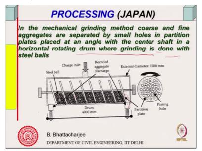
In the mechanical grinding method coarse and fine aggregates are separated by small holes, right? In a partition plates I will show the diagram placed at an angle with center shaft, with center shaft in a horizontal rotating drum where grinding is done with steel balls.
