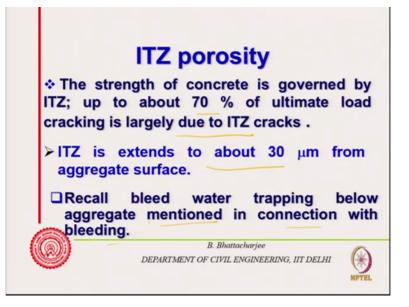
So that is what it is pores, now my problem why, what is role (())(14:51) aggregate, yeah that is call recycled aggregate, that is got a role. The strength of the concrete is governed by ITZ upto 70 percent of the ultimate strength and cracking is largely to ITZ cracks.
