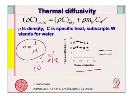
Now this one is thermal diffusivity of volumetric heat capacity. It is a simple additive property. For example, if I have (mois) if I have some moisture, some theta degree of saturation then it will cause increase in the moisture content and mass will increase by the amount of moisture, so supposing I am trying to find out the mass per unit volume, density.
