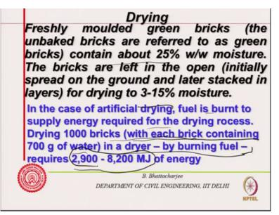
Then this is drying freshly molded green bricks they have you know the unbaked bricks are referred as green bricks. So they are not anything greener but in the terminology, similar terminology we are using also for concrete green concrete, plastic concrete earlier we were using. Not the green today we understand, so referred as green bricks contain about 25 percent moisture roughly than they are left in open for drying. And stacked to reduce it down to 3 to 15 percent moisture content.
