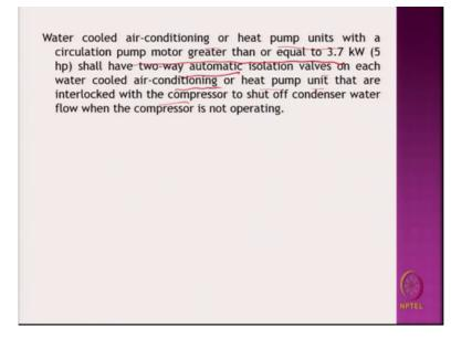
Water cooled air-conditioning or heat pump units with a circulation pump motor greater than or equal to 3.7 kilo Watt shall have two-way automatic isolation valves, water cooled air-conditioning or heat pump unit that are interlocked that is if you both act together then you should have isolation valves so one goes other does not work.
