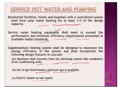
Similarly, such prescriptive requirements are also given for service hot water and pumping that means these are mandatory requirements even when you have trade off option. So, centralized system shall have solar water heater minimum at least one fifth of the design capacity should be through solar heat water.
