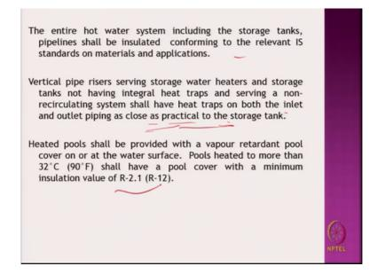
The entire hot water system includes storage tanks, pipelines that as per design and you know shall have heat traps on both the inlet and outlet and heated swimming pools if they are there shall be provided with a vapor retardant pool cover. So, minimizing the loss and pools heated to more than 32 degree centigrade shall have a pool cover with a minimum insulation of this. So, these are the mandatory requirements given.
