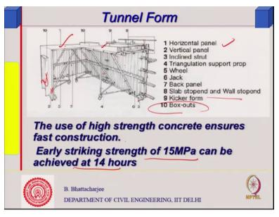
This is what it looks like, so if you look at it there are horizontal panels so these are horizontal panels, make the floor bottom of the floor, bottom of the floor right bottom of the floor. Then vertical panels, so vertical panels are this one. Concrete will come on the side, concrete will come on the side, concrete will come on top of this. Incline struts so these are inclined struts which will support the foam and
