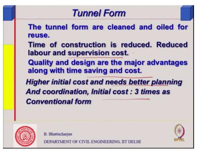
So tunnel form a clean and oiled for the reuse. Time of construction is reduced, reduced labor and supervision cost, quality and design are the major advantages along with time saving or cost, initial cost is higher. In all this initial cost is a little bit higher. Better planning and coordination. You know initial cost can be 3 times than conventional form. (Refer Slide Time: 28:26)
