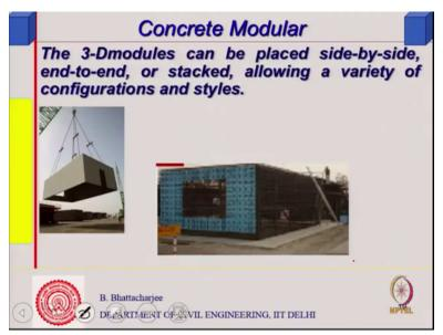
So that is what is tunnel form I think we will stop it here, and we will look into concrete modular in the next case and I will not going to this, so this you can understand it is a modular box, complete box, modular box and you can built lot many things in this so this is 3D modular system and we will look into some similar advance industrialized construction in the next class.
