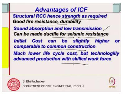
So, structural RCC hence strength is strength as required. Now fire resistance, the insulation material normally and not good fire resistor, thermocoal will simply you know they will, in fact they will add to the fire load. They are carbonaceous material they will add to the fire load, they are good insulation. So you have something the finish itself has to be fire resistance kind of finish that would be there on top.
