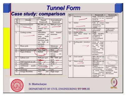
So somebody has done a case study in India and this case study is very interesting. Procurement cost was 22,000 per square foot I mean square meter for this one. Conventional 800 per square meter, so you can see 800 to 22,000 not 3 times is much higher. Casting system, monolithic etc etc RCC framed structure and this is monolithic slab and etc, floor 1 to 3 days this requires 3 to 4 weeks.
