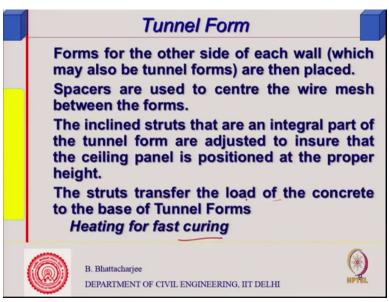
So either side you know then placed ok etc. Heating and fast curing as a struts, struts actually transfer the load of the concrete to the base of the tunnel forms.
