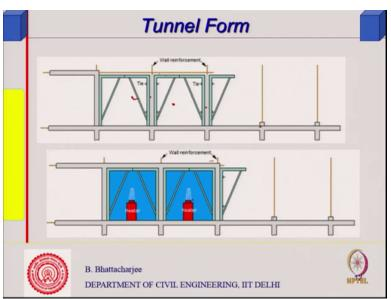
So this is already existing floor and so on, then there must be heating, so heating in order to get it fast cured. And the slab reinforcement then you put in, first is the wall reinforcement, then slab
