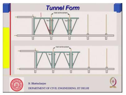
And this how it is, so this is what is cast already now this will be cast the tunnel form has come this maintains the you know this this actually carries the load, transfers the load to the from the slab to this and to the bottom kind of a bracing and then putting the reinforcement, reinforcement, reinforcement the concrete comes in and here is a concrete has now come in wet concrete, it has come in here. The rods of course protrude out for the next level and so on.
