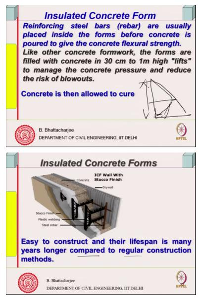
Now pressure on the formwork is something of this kind. Pressure on the formwork is something of this kind hydrostatic is not exactly hydrostatic pressure. That like this you know so fresh concrete does not offer hydrostatic pressure as such. Why? Because the time you pour it sets some amount of setting would occur, so the bottom concrete it can withstand on its own, so you
