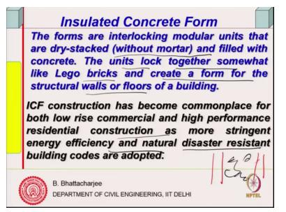
These forms are interlocking modular units. This, you know the forms are interlocking modular units that a dry stacked, without water stack them up and filled with concrete. For example, if you have Polystyrene, expanded polystyrene. Expanded polystyrene here, expanded polystyrene here. And then fill in concrete material here and this remains, obviously they will need some finishing on top of that. You need some finishing on top of them.
