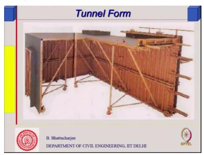
So that is how it looks like the same one photograph, so here the concrete will come and here the concrete will come, here the concrete will come, this is the portion which is supporting the slab part of it.
