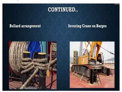
This is the bollard arrangement as you can see so it has to be tied in a particular pattern. So that hankering can be done properly structural materials supports winches or cranes shall be in a good condition and fully secured over the barge. As you can see in this particular picture, we have crane mounted on a barge and how it is secured properly using structural steel material. Crane swing area should be marked and warning signs shall be placed.
