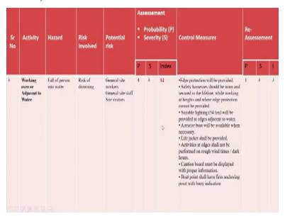
Now we have another activity the working over or adjacent to water, this is one of the most important things in any port and harbor construction. Because this is mostly done for over 50% of the project work so what is hazard? Hazard is fall of a person into water. Risk is risk of drowning. Potential risk everybody who is working on that particular area is potential risk. So, what is the severity and probability?
