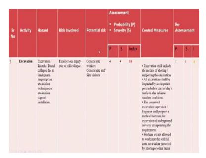
Next activity we have is excavation. So here also hazards risks potential risk factors established to a little; severities are given and control measures are established. So, what are the control measures? Excavation shall include the method of shoring the excavation all the excavation shall be inspected by competent person before start of the day's work. So, you can see if these control measures are established the risk index can be brought from 16 to a 4 value.
