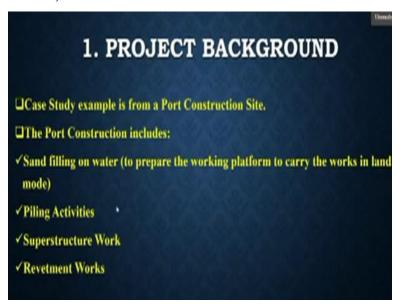
So, the case study that I have taken is from a port construction site. So, port construction basically includes following things done. One is sand filling on water, pilling activities, superstructure work, revetment works. So, what is sand filling on water? So, this is basically done to prepare the working platform so that most of the works can be done on a land mode of construction. And it becomes easy to construct anything on a land as compared to water.
