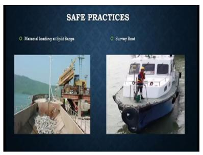
On the left you can see this is a material loading activity going on at a location where the dumper or the truck you call is unloading the rocks into a split barge. This is also kind of a barge which is used for transporting a, materials from one place to another. So, you can see here as edge protection given here for this particular kind of activity. On the right-hand side, you can see a survey boat.
