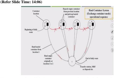
Now suppose the vehicle has one empty container. So before starting from their beginning location, they will have one empty container. So what the vehicle will do, that will go to the first container location. It will deposit the empty container and the full container will get hauled to the disposal site or recycling facility. Now the vehicle in this case again will have one empty container.
