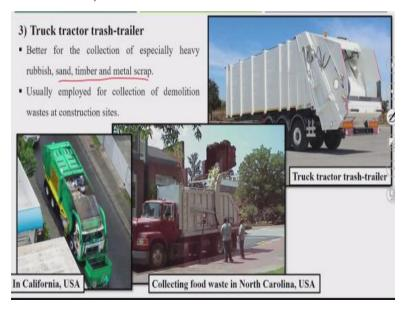
Now next is the truck tractor trash-trailer. Now here as you can see, one special trailer is available in this vehicle. So that is specially used for the heavy rubbish, large size material, the sand, timber, the metal scrap. Especially for the collection of inert material
