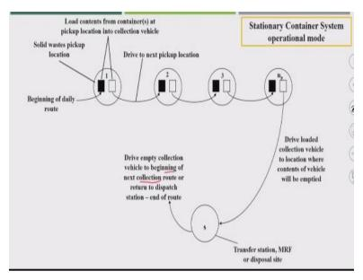
Now, another example of this stationary container system. Similarly, if we have "n" number of container locations and one disposal site or transfer station is available. Now the vehicle will start the daily route. It will go to the first location and will load content from the container at pickup location into the collection vehicle, okay. Because here container is not getting loaded.
