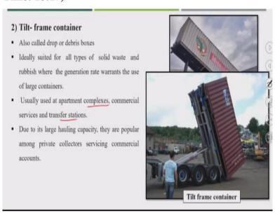
So you see. Here is a tilt frame container that can rotate up to 80 degrees angle.
