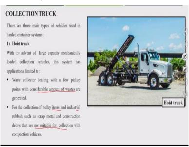
Now there are different kinds of collection vehicles used to be used for the haul container system. There are three main types of vehicles. First is the hoist truck. You see in the photograph of the hoist truck. However, the application of mechanically loaded collection vehicles with large capacity is limited for the areas where a considerable amount of waste is generated.
