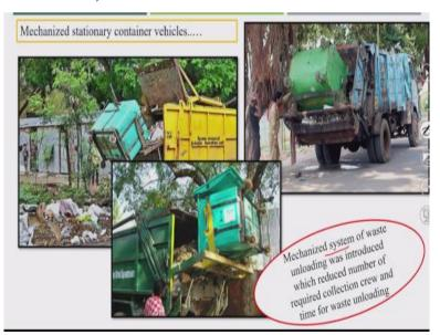
And along with that, some cities did not start the haul container system. They were with the stationary containers only. So in that case, only the waste used to be emptied into the vehicle. So, later mechanization had been started because the time required for loading the vehicle was very high, and these kinds of vehicles used to be on the road causing a lot of traffic problems.
