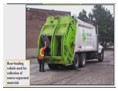
This is rear loading, the backside loading.
