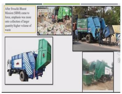
Now after Swachh Bharat Mission, this same stationary container system had been changed into the compactor vehicles. You see here some of the photographs you can see. As earlier, the vehicle volume was very small and the vehicle used to be able to collect only one ton or at the maximum two tons of waste per trip.
