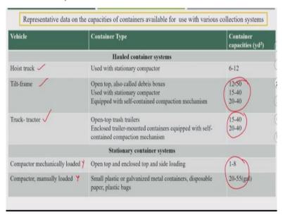
Now here, one more comparison can be made among the containers available for use with the various collection system. As you can see, I have assigned different types of containers for different types of vehicles. These three are for the haul container system. And these two are for stationary container system. So here see the capacity. Here especially the tilt-frame, the capacity is very large.
