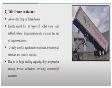
Now, this another vehicle that is called a tilt-frame container. Now, in this case, you can see the entire back frame is getting tilted. Unloading is very easy from this kind of vehicle. So, this is ideally suited for all types of solid waste, rubbish where the generation rate warrants the use of the large container. So wherever the waste generation is very large you can have this big size of the container.
