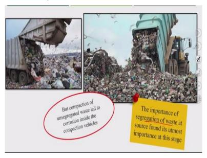
But the problem with these compactor vehicles was that, as unsegregated material was getting compacted, so obviously when it is 40 to 60% of biological content used to get compacted, obviously there used to be the release of a lot of moisture. And this spillage or leachate, whatever was coming out the after compaction of this waste used to be highly corrosive with pH normally in the range of 3 to 4 i.e. acidic.
