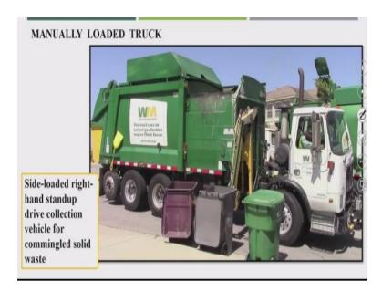
So you will see here, a side loaded vehicle. Here loading is done manually sideways. So these containers are getting unloaded into the vehicle. We get a mixed waste here. However, even segregated waste also we can have two different locations where dry waste, the wet waste we can segregatedly we can load it into the vehicle.
