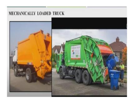
As you can see here, the truck is getting mechanically loaded. Earlier, we saw a truck with a manually loaded facility. Now here, we can see rear-loaded mechanically loaded loading facility.
