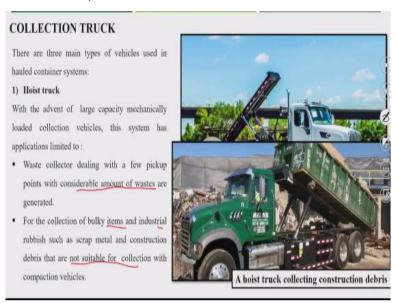
See here another hoist truck collecting construction debris.
