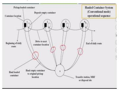
So this is one example I am giving how the haul container system will work. Suppose, you see, here are the locations. So I put the containers in the first location, second location, third, and so on. Likewise, there are "n" number of locations of dustbins or containers inside the city. So a city could have say, 300-400 different dustbin locations. And there will be a one finally where the entire waste or these containers are getting transport to either transfer station MRF or disposal site.
