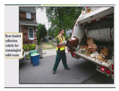
Here is a manual loading or mixed waste from the rear-loaded collection vehicle. And it is having the compaction facility, the waste is getting compacted.
