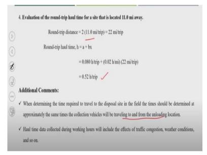
So evaluation of the round trip haul time for a site that is located 11 miles away. So first we have to calculate round trip distance i.e., x value which will be double of whatever the distance is given for the locations. So  $(2 \times 11) = 22$  miles per trip i.e., round trip distance. Now, we will calculate the round trip haul distance h = a + bx; a and b we found. And we will multiply by x.
