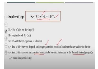
Now here another equation to calculate the number of trips, that is  $N_d$  that number of trips in a day. That normally finds how much time available in a day this is how much time available in a day and how much time is required for one trip. In that way, we can calculate the number of trips. Now here, you see here the time available in a day we calculate it like we minimize the off-route time.
