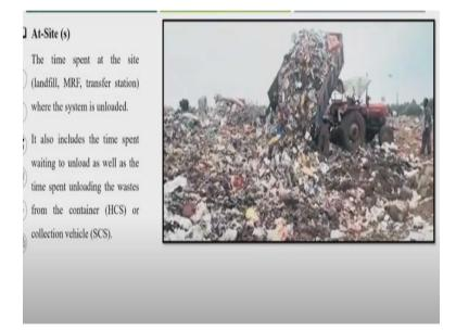
Next is the at-site time. This is the time spent at the site. That is the final place where the waste is getting disposed off. That is that could be a landfill, MRF (Material Recovery Facility), or transfer station, where the system is unloaded. So that time also includes the time spent waiting to unload as well as the time spent unloading the waste from the container or collection vehicle in both cases.
