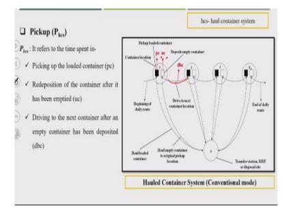
So you see here the first is the pickup time or that nominated by  $P_{hcs}$ . Here "hcs" is a named as haul container system, okay. So now here, this is what we see that the flow of the vehicle in a different location. So what will the pickup time or pickup unit operation? That picking up a loaded container. So that is you see here pc that we normally called as a pc picking up the loaded container.
