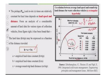
Now next is the pickup time, at-site time. Even at-site time is known how much time will be required to empty the container at the disposal site or recycling facility are relatively constant. Almost you know that how much time will be required in that case. But the haul time depends on haul speed and distance. What is the distance from that particular location from different locations, what is the distance and also the speed is also important to find out the haul time.
