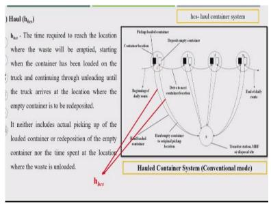
So the next functional unit operation is a haul. That is the time required to reach the location where the waste will be emptied and starting when the container has been loaded on the truck can continue through unloading until the truck arrives at the location where the empty container is to be redeposited.
