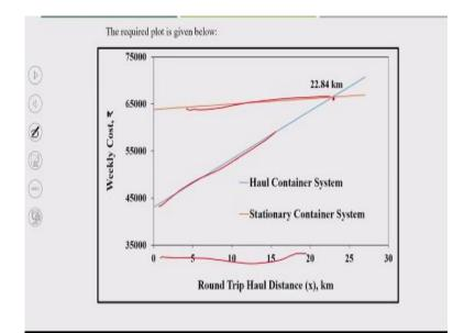
So we plotted this graph between the round trip haul distance versus weekly cost. And surprisingly you see the graph here the haul container system for initially for up to around 20 kilometers the total cost for haul container system was lower than the stationary container system and at the point, 22.84 kilometers the cost of haul container system and stationary container system will be the same cost will be required.
