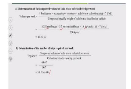
Now we will see the determination of the compacted volume of solid waste to be collected per week. So then we know that volume per week, we can calculate by residence into occupants per residence multiplied by solid waste collection rate and multiply by 7 days in a week, okay? Because once in a week collection facility. We will divide by the density or specific weight of solid waste in the collection vehicle.
