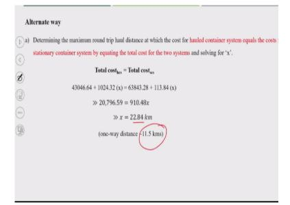
But there is an alternate way we can easily we can calculate the x value. If you put both the values the same as the total cost of the haul container system is the same as the total cost of the stationary container system. By that way we can come up with the x value; x also here the same value is coming 22.84 and that one-way distance of 11.5 kilometers is the answer to the problem.
