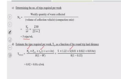
Now we will determine the number of trips per week that  $N_w$  value okay first. That we can calculate by the weekly quantity of waste collected divided by the volume of container vehicles. Is also a very simple number of trips required per week can be calculated if you know that the weekly quantity of how much quantity of waste collected is divided by the volume of the collection vehicle. Only we multiply the compaction ratio with that.
