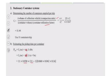
So for the stationary container system, first we determine the number of containers emptied per trip that is C t value. So this we can calculate by volume of collection vehicle divided by container volume. This is simply we can calculate the number of containers emptied per trip. If you know the volume of the collection vehicle and if you know the container volume.
