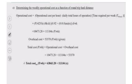
Now we will determine the weekly operation cost is a cost, which is a function of round trip haul distance. So in the same way, we can calculate the operation cost, per hour cost multiplied by the daily hour of operation and multiplied by  $T_w$  value for stationary container system. The same way it is calculated and it comes to be (10,473.28 + 113.84 x) Rs./week. So overhead cost, again the overhead cost is already given here.
