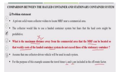
So we will directly go to the problem. And the problem statement is, a private solid waste collection vehicle locate to the MRF a material recovery facility or recycling facility near a commercial area, okay, one private waste collector. And the collector would like to use haul container system but fear that the haul cost might be prohibitive.
