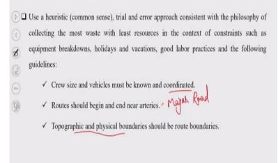
So the collection route uses a heuristic method or we can say is common sense, based on common sense. Or also can say the trial and error method, what corporations used to do. Approach with the philosophy of collecting the most waste with least resources in the context of constraints such as equipment breakdown, holidays, vacation, good labor practice, and another few more guidelines, okay.
