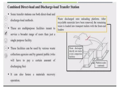
Now the third type is combined direct-load and discharge-load transfer station facility. So is a combination of both direct-load and discharge-load. So these are multipurpose facilities meant to service a broader range of users that just is a single-purpose facility. So now here there are two different facilities. So, I personally believe that this kind of transfer station is always beneficial for India.
