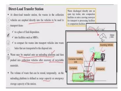
So here you can see here, this is the incoming vehicle, the smaller size of the vehicle is getting unloaded into the larger container. This is the container of large vehicle and it is having one facility of compaction. The waste is getting unloaded, it is getting compacted and this compacted waste is going to the larger container. So this kind of facility could possible.
