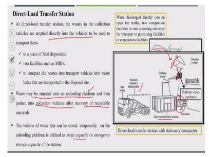
So here you can see this is the truck from waste is getting collected and here is getting unloaded and here maybe here one compaction facility also could be possible and this is the large container transfer station. This will get hauled to the disposal site or recycling facility. So the volume of waste that can be stored temporarily on the unloading platform is defined as surge capacity or the emergency storage capacity of the station, whatever the maximum capacity of that particular station.
