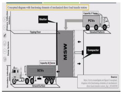
So this is another one more photograph, simple. So here are 3 tons capacity of one vehicle. The MSW is unloading, here the compaction facility and another vehicle having the larger container which can take 20 tons of waste in one trip.
