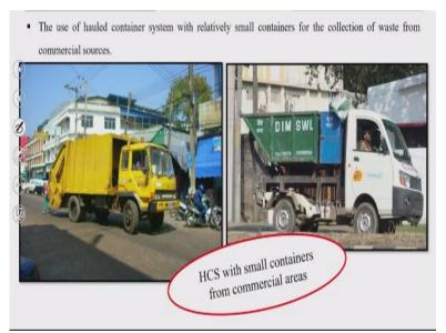
Now, this another benefit that the use of haul container system with relatively small containers for the collection of waste from the commercial sources. Now normally in the commercial areas normally we have to use the stationary container system and the quantity is very large and very difficult to have haul container system because the size of the vehicle will be somewhat large.
