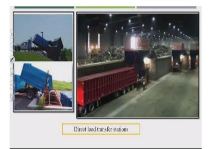
So you can see here this is very simple facility. Waste is getting hauled and this is the bigger container is here, okay. This is another facility. So here waste is getting first deposited into the floor and after that is getting unloaded into the larger container.
