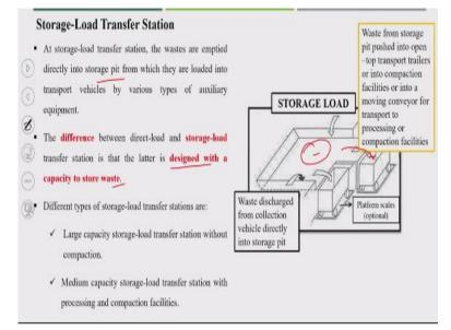
Now next is the storage-load transfer station. So here the name just signifies storage facility. Means waste is getting stored and then it is getting loaded onto the larger vehicle. So at storage-load transfer station, wastes are emptied directly into a storage pit. So it is getting unloaded into a storage pit which they are loaded into the transport vehicle by various types of some different auxiliary equipment.
