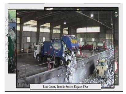
So here are also the this is one of the photographs from the US. The waste is getting unloaded into the storage pit.
