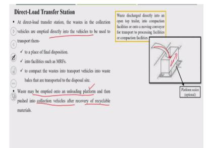
First, we will see the direct load transfer station. So at the direct load transfer station, the waste in the collection vehicles are emptied directly into the vehicle to be used to transport them to a place of final deposition directly emptied directly into the vehicle and transferred to place of final deposition into facilities such as MRF facilities it will go. Or to compact the waste into transport vehicles, the waste bales are transported to the disposal site.
