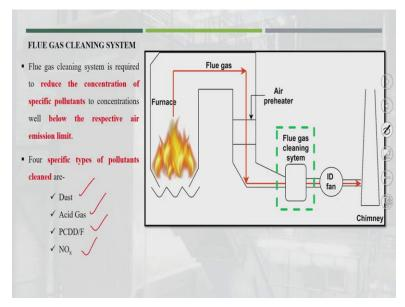
Now we will talk about the flue gas cleaning system. So normally was from furnace flue gas is produced that will go to the flue gas cleaning system. Ok. so, flue gas cleaning system requires reduction in the concentration of specific pollutants consideration well below the respective year emission limit we saw in the previous slide, and there were four major pollutants.
