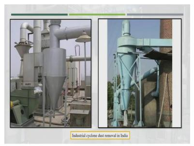
This is an industrial cyclone dust removal in India. Next unit is the electrostatic precipitator. (**Refer Slide Time: 15:23**)
