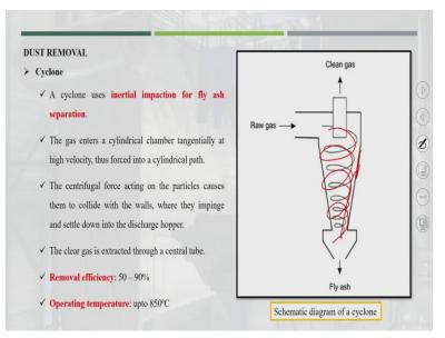
The first quality is the dust. So how the dust is removed? so, there are different kinds of treatment facilities available for the dust removal. The first is the cyclone. so cyclone on uses inertial impaction of the fly a separation like you see here is a one of the line diagram of the cyclone. So the flue gas is getting like waves passing through this particular vertical unit. So the gas enters a cylinder chamber tangentially at the high velocity that force into a cylindrical path.
