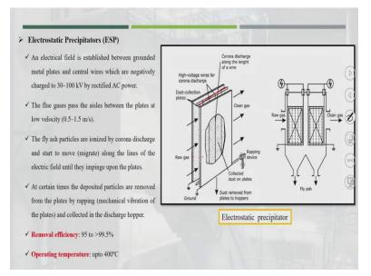
This is one of the oldest treatment unit for removal of dust particle. The small size particle, fine particle also can be easily removed from the electrostatic precipitator here in the ESP the electrical field is established between the grounded metal plates and central wire which are
