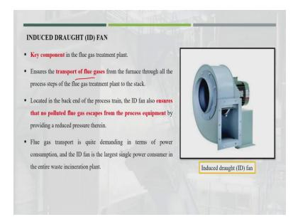
So these ID fans called induced draught fan, see here is the draught fan. You see in the previous slide; it is put in the last. So, whatever gas is produced from the furnace, how that gas will go to the treatment system or how we can maintain the velocity, whatever velocity is required through cleaning system, and again that gas has to go to the stack, so this management is entire by the ID fans. So ID fan this is the end of this treatment system.
