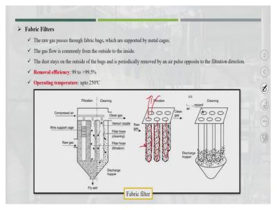
It is another technology or another treatment technology. It is available to remove the particles of dust? The raw gas passes through the fabric bags which are supported by metal cage. So this is the fabric bags, and the glass floor in commonly from the outside to the inside. So from outside to inside and finally from this the clean gas will come out. The dust is on the outside of the bag and periodically removed by air pulses opposite to the filtration direction.
