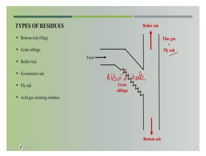
So suppose this is the furnace and this is the grate. So first we will be the bottom ash, so once this is the bottom ash, so once the feed will get combusted on the grate. So the combustible material for non combustible matter will be come out in the form of bottom ash that we can say is in slag also. Next is the grate sifting, so the grate sifting is coming out from the openings in the grate.
