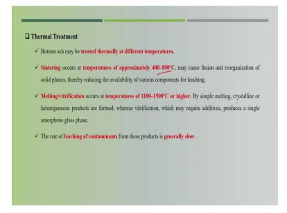
Next statement is thermal treatment. So bottom ash may be treated thermal at different temperature because if you see the calorific value of these ashes also is very high. So also could be combusted again or sintering occurs at temperature of approximately 400 to 850°C mainly causes fusion and reorganization of solid phases thereby reducing the availability of various components for leaching.
