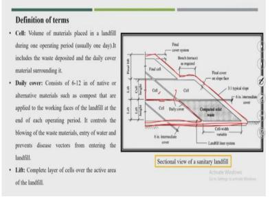
So, now, if you define the different terms, this is the 1 sectional view of the sanitary landfill. So, and you see here different words I wrote it, which I am going to explain here. So, the first is cell. So, you see here cells, there are different cells. So, here I think this is the crosssectional of the landfill area, this is the top area of the landfill and this is the ground. So, , what is cell? This is the volume of material placed in a landfill during the 1 operating period usually 1 day.
