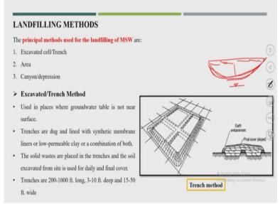
Now the landfilling methods, so, there are 3 major methods of landfilling, or we can call as a there are 3 types of landfills. First is the excavated cell or trench method. Next is the area method and the third is canyon or depression method. So, first is an excavated or trench method, this is the most popular method of landfilling. So, this name just you can understand is excavated.
