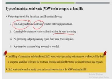
So, the type of municipal solid waste to be accepted at the landfill so, the waste category is suitable for sanitary landfill are as following you see here I put it there are 4 kinds of waste should come to the landfill area. The first is non-biodegradable and inert waste by nature or through pretreatment. So, this is what whatever is non-biodegradable or inert waste that will come to the disposal site or landfill site, the commingled waste mixed waste not found suitable for waste processing.
