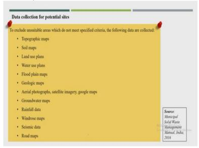
Now the data collections so what kind of data has to be collect in that potential sites, topographic maps, soil maps, land use plan, water use plan, floodplain map, geological map, aerial photograph, groundwater map, rainfall data, windrose map, seismic data, roadmaps these data need to be collected for the all potential site and important which I found that the groundwater map, rainfall data this is the important one, even roadmaps also is very important to reach to that particular locations.
