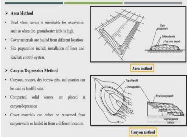
Now, next is the area method. So used when the terrain is unsuitable for excavation, such as when the groundwater table is high. Now, in the same example, suppose this is our surface and now the water table is somewhere here. Now, in this case, suppose if you go for excavated cell method or trench method, so, if you go for excavation like this, so, obviously, your entire disposal site will be in the flooded area, so, it is very difficult to dispose the waste into such cases.
