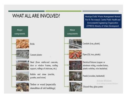
So what all is involved here is the significant components and minor components like major components are brick, cement plaster, steel or maybe stone, granite and wood or timbers. These are the essential components in the C and D waste. A few minor features like conduits like iron could be possible the pipes, electrical materials, the panels, or even glass panels could be likely. But I think this is a minor component, but major are these are the major ones.
