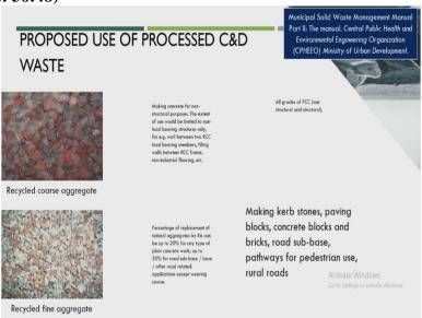
So again, these kinds of coarse aggregates and fine aggregates to make concrete for nonstructural purposes. Also, all grades of PCC could be made out of these aggregates percentage replacement
