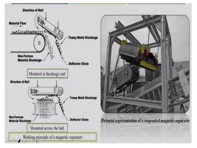
This is a magnetic separator. Like here one another magnetic separator. So from that, the magnetic particle is getting separated from the main waste.
