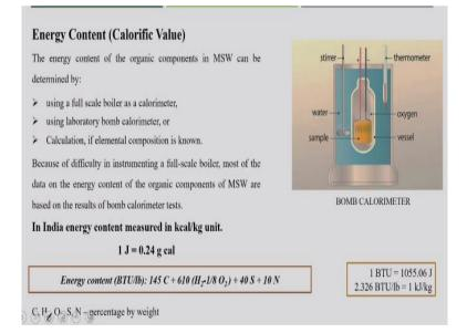
There is another parameter called energy content or calorific value. This is normally designed by a full-scale boiler as in calorimeter or laboratory one bomb calorimeter. This is one small diagram of the bomb calorimeter. In a vessel, the waste is getting combusted. And normally this energy content we calculated by this formula having the concentration of carbon, hydrogen, oxygen, sulfur, and nitrogen.
