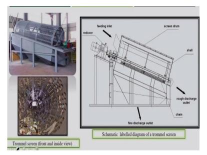
So and these are the few machines normally or equipment we use to separate the different sizes of the particle. Like this is Trommel. This is simply one of the other Trommel screens.
