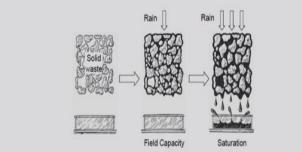
So this is another physical parameter is the field capacity. This field capacity is the total amount of moisture that can be retained in the waste sample subject to the downward pull of gravity. This parameter is very important to know about how much leachate is getting produced once the waste goes to the disposal site. So is an excess of the water over the field capacity will be released as leachate.
