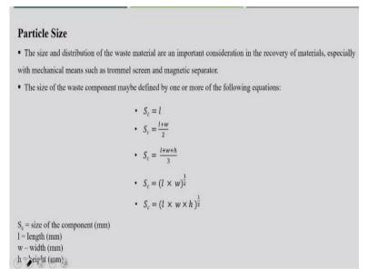
Another parameter is called particle size. These parameters normally are important for the recycling facility because there we need to know what kind of size. Even for the degradation process also we need to know the particle size. There are different ways of calculation of particle size like there are different ways based on the length and width or height of that particular material.
