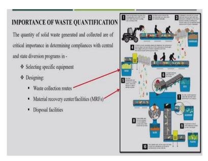
Also for the MRF facility or Material Recovery Facility, whether it is a recycling facility or any biological treatment facility, quantity is very important to know about the manpower requirement or resource requirement. Even the land requirement for supposing for compost plant if you are designing and if you do not know the quantity is very difficult to finalize how much is the land will be required for the composting facility.
