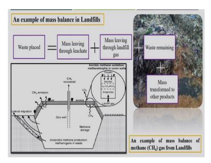
So there is an example of mass balance in the landfill. So how to calculate the waste placed into the landfill. That we can measure that mass leaving through the leachate. So the leachate is getting produced. So if you know that how much is the leachate is getting produced into the landfill site that will include plus the mass leaving through the landfill gases.
