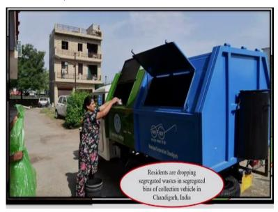
Here, you can see under the Swachh Bharat Mission collection vehicle has been used for waste collection where a green bin is used for wet waste, and a blue bin is used for dry waste. For household hazardous waste, an everyday yellow bin is not provided since waste generation is not very large. It is mostly collected once in a week or two times in a week or alternate days of the week.
