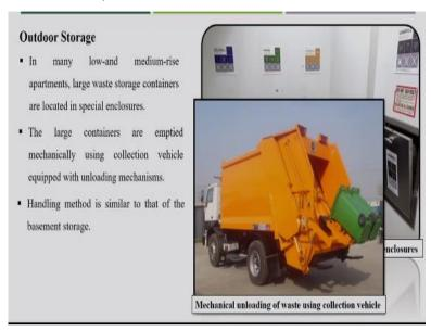
Like here this mechanical unloading of the waste from using a collection vehicle can be possible.
