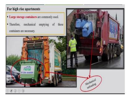
For high-rise apartments, a large storage container is commonly used. Here, the curb service is very common and generally mechanical unloading is done to empty the waste into the collection vehicle, which can be seen here.
