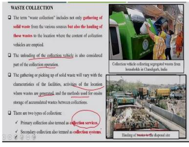
And finally, from the treatment sites or transfer station, it will finally go to the disposal site. So here, unloading of the collection vehicle is also considered collection operation okay. This is to be understood that, not only the collection from the source also the unloading of these vehicles and the transportation from one location to another is also included in the collection process.
