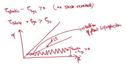
Similarly, another case can be there where tau static minus tau cyclic is still greater than 0. So, that means no stress reversal, but tau static plus tau cyclic is more than the steady-state shear strength. So, what will happen in this particular case? The initial state of the sample was like this, but when it is subjected to cyclic loading, the sample reaches the flow liquefaction surface. In addition, this particular point will again be called the initiation of flow liquefaction. So, in
