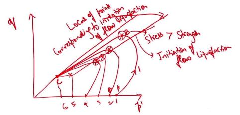
So, one example is shown over here. Similarly, we can repeat the same thing, and we will have what we will get each of these samples. That means, we are repeating the test on very loose
