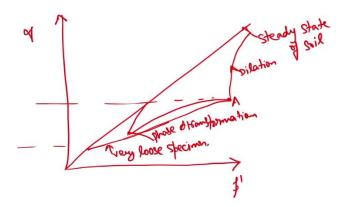
So, here, we can see the sample is going up to—this was the state which was identified as the steady state of the soil. Steady state of soil. That means, samples considering the initial state of
