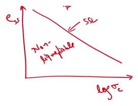
This plot corresponds to the steady state line, where liquefiable soil is on one side and non-liquefiable soil on the other. Whether the soil will undergo liquefaction depends not only on this but also on the stress path. The nature of the loading is also significant. As I mentioned, the nature of the loading helps understand the triggering mechanism, particularly the initiation of flow liquefaction. This can happen during monotonic loading, including in natural soil
