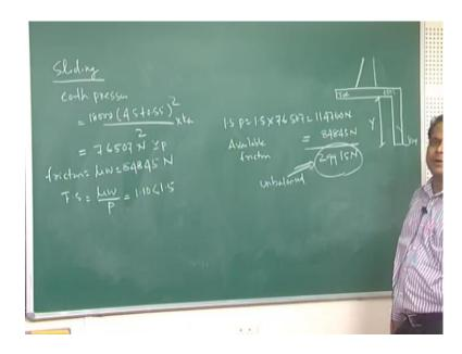
So, total horizontal earth presser earth presser, now this is for check for sliding earth presser is coming about to be eighteen thousand in to 4.5 plus zero 0.554 0.5 how it is coming this distance is your 4.1 plus zero point four this is your 4.5 plus this site is your 0.55. So, this hole square by two in to k a, and this value is coming about to be 76507 Newton. So, maximum fiction how much fiction your getting the fiction is coming about to be me w, and this is equal to 84845 Newton.
