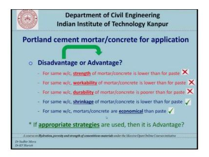
Now, let us move to Portland cement mortars or concrete when we are saying for application now the same slide if you see from the standpoint of mortars what we have is that for the same mortar to cement ratio strength of mortars or concrete is lower than paste and likewise for workability and likewise for durability. So, the negative that you have in mortars or concrete is primarily because of the use of fine aggregates and coarse aggregates in proper proportions.
