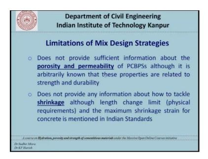
At the other limitation is that mix design strategies does not provide sufficient information about the porosity and permeability of Portland cement based paste systems although it is arbitrary known that these properties are related to strength and durability.
