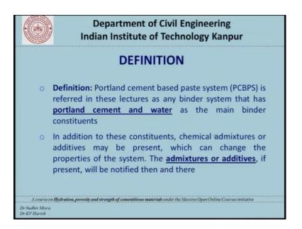
So, definition Portland cement based paste system we are referring in this lectures as any binder system that contains Portland cement and water as the main binder constituent that does not mean that the binder constituent should only have Portland cement and water it may have some admixtures or additives or chemical admixtures. So, the presence of these admixtures additives can actually modify the Portland cement or Portland cement paste.
