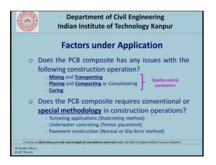
So, what we have seen here is that under application depending upon the construction operation or the special methodology used or situation specific or special requirements the factors keeps on changing and for different application we have different set of factors that come into picture and this is primarily important when you go for the selection of a particular Portland cement based paste systems.
