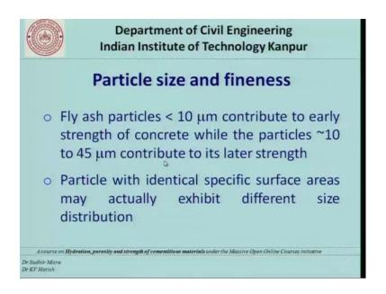
Now, fly ash particles lower than 10 microns this is a very important point. Fly ash particles lower than 10 micron contributes to early strength of concrete. Remember that the early strength of concrete in Portland cement based phase system is primarily
