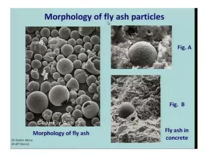
So, what is meant by morphology? Morphology refers to primarily to the shape of the particle. So, fly ash particles are spherical in shape that is a very important point, because in the naked eye we cannot really see whether it is spherical or not. Only in under
