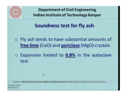
Now, the second one is soundness test where we have not getting in to the soundness test because it is already discussed in Portland cement. All that you have to know is that the soundness problems may exist if fly ash has higher quantity of free lime or magnesium oxide crystals and the limited expansion values are 0.8 percentage in the autoclave test.
