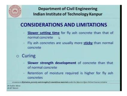
In addition to that other problems such as slow setting time. So, when you use fly ash we have already seen that it increases the setting time. So, and not only that on the other hand it also produces a sticky mixture. So, sometime these scenes create problems while mixing and placing operations.
