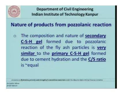
Now, getting into what are the nature what is the nature of product from pozzolanic reaction, we have already seen what is pozzolanic reaction. And we know that calcium silicate hydrate gel is basically formed because of the reaction of pozzolan and the calcium hydro oxide that is formed from cement hydration.
