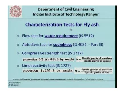
So, there are typically 4 characterization test that are mention in the Indian standards. One is the flow test. And flow test is primarily for water requirement. And it this is specified in IS 5512 and what is mean by flow test how the flow is measured and all those things we will see a little later.
