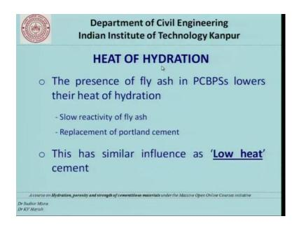
Now, the next property is heat of hydration. The presence of fly ash in Portland cement based paste system lowers their heat of hydration, very important point and this is one reason why in structure where heat of hydration is a very critical factor fly ash is used as a very important material in concrete. So, why a because number one the reactivity of fly ash particles is usually slow. So, they do not react within 2 3 days they take their own time to react probably in 7 days 14 days or 28 days.
