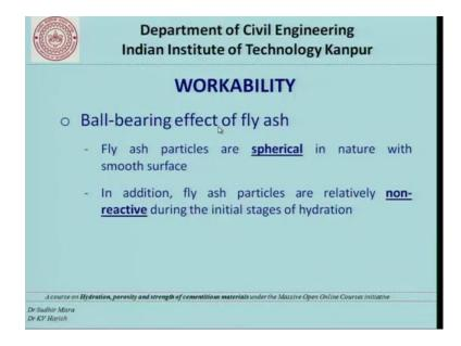
The other one is ball bearing effect. So, the word ball bearing effect is to indicate that the fly ash is spherical in shape. And when you have a smooth spherical shape then the particle to particle interaction is much lower and this actually helps and the additional thing is that the fly ash particles are non reactive at early stages.
