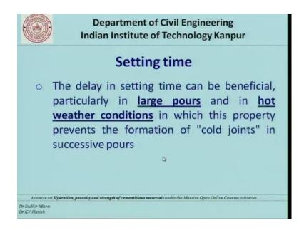
Ah factor when it comes to large volume of concrete. So if you take an example of dam or other structure where huge amount of concrete is used this, this point is very much valid the delay in setting time can be beneficial particularly in large pores and in hot weather conditions in which this property prevents the formation of cold joints in successive pores.
