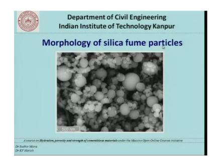
So, a scanning electron microscope image is shown where you can see that at a 500 nanometer level we can see that the shape of the silica fume particles are spherical. And remember that this is 500 nanometer is 10 power minus 9 meters. And what we also see is the agglomeration that is few particles together join I mean particles together join with each other and they are generally seen as agglomerated or condensed or densified form. So, that is what is can be observed from this figure.
