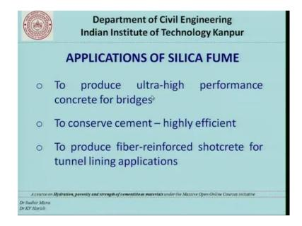
The other application is as already mentioned; silica fume can be used at a much higher dosage in ultra high performance concreted for bridges. And sometimes if it is specified that the quantity of cement is substantial and it creates higher reactivity in the in the in that particular application. Silica fume can also be used to conserve cement or to reduce the use of cement. The final one is a silica fume can also be used for fiber reinforced shotcrete applications primarily in tunnels.
