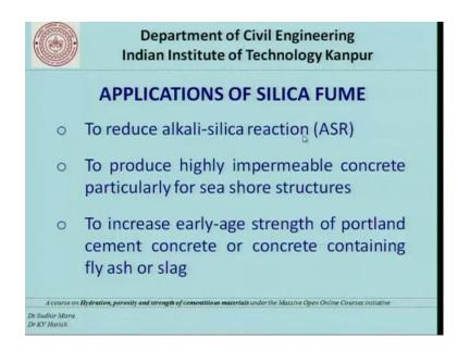
Applications of silica fume. Silica fume is primarily used to reduce alkali silica reaction. It is a very effective pozzolone and the alkali silica reaction problems are largely encountered by using silica fume at very low dosages. Even fly ash is capable of reducing expansions, but not to the level silica fume reduces.
