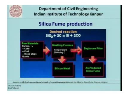
Now, more information about what are the raw materials that are used in the silica fume production and others. Raw material such as carbon and quartz are used and the primary source of carbon is coke coal or wood chips. And primarily they are subjected to very high temperature a this melting furnace usually it ranges from 1800 degree Celsius to about 2000 degree Celsius.
