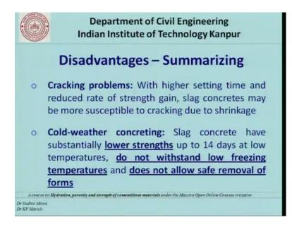
So, this is about advantages that does not mean that you do not have disadvantages. You also have disadvantages such as cracking problem especially because of the lower because of higher setting time and reduced rate of strength gain and others.
