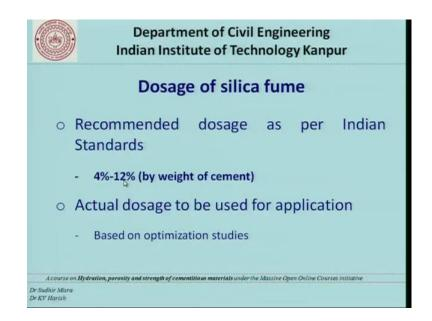
So, the recommended dosage typically varies from 4 to 12 percentage and remember that this is by weight of cement when you replace it by weight of cement and another information is that this is as per Indian standards.
