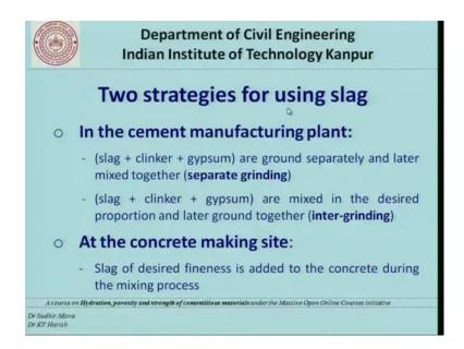
The 2 strategies that are used while using slag are as follows. Slag can be either added directly in the cement manufacturing unit. Or it can be used at the concrete making side it directly as a admixture in a concrete.
