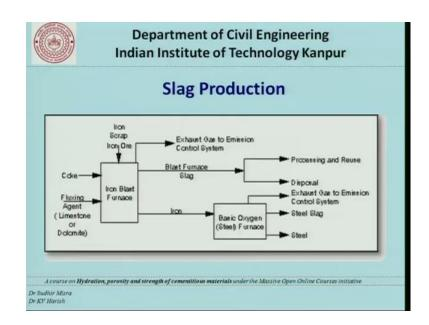
The coke or limestone or dolomite which are actually the raw materials for iron, and again you may have some iron source which are added as a scrap material into the furnace and you get the iron the pure iron and you also get slag and again this slag can be either disposed or this can be processed and reuse and again in this iron you have the basic oxygen furnace through which steel is produced.
