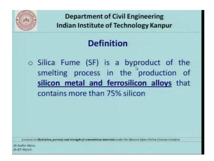
So, we will now start with silica fume. So, production of silica fume first of all definition what is meant by silica fume. Silica fume is a byproduct of the smelting process in the production of silicon metal and ferrosilicon alloys that contains more than 75 percentage silicon. So, by definition silica fume is a byproduct in the production process of silicon metal and ferrosilicon alloy.
