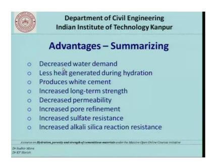
So, these replacement levels are at recommended replacement levels. Now summarizing some of the advantages of slag. Slag decreases the water demand. Less heat is generated during hydration. It also produces more whitish cement in addition to that it also has increased a long term strength, decreased permeability, increased pore refinement which means a smaller pore size, increased sulfate resistance and increased alkali silica reaction resistance.
