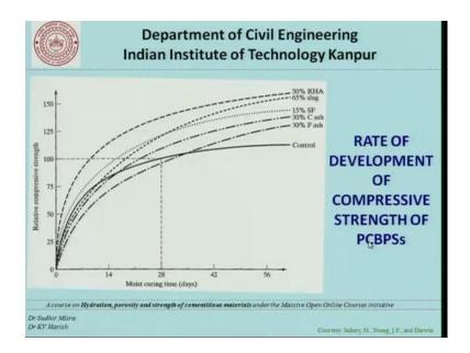
Now, coming to the rate of strength development graph, if we have to compare it with the other admixtures like fly ash and in specific class C or class of fly ash the figure is shown remember that this is a revisiting figure in the sense that we have already seen this in fly ash the same figure is shown just to compare how silica fume mixture performs compared to a fly ash mixture or control.
