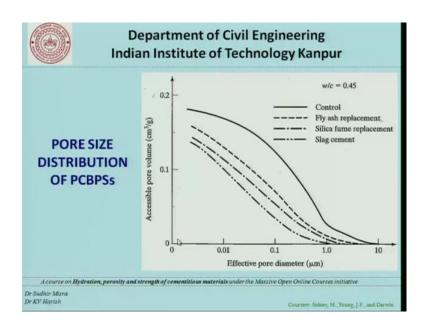
The next property is pore size distribution and what we find in this figure is that you have effective pore diameter in the x axis ranging from 0 micron meter to approximately
