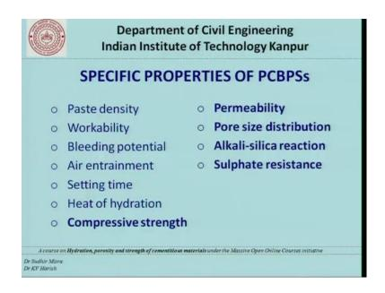
Some of the properties that we are going to see or page density workability breeding potential air entrainment, setting time heat of hydration compressive strength permeability, pore size distribution, alkali silica reaction and sulphate resistance remember that many of these properties have been already seen for fly ash. So, now, we are actually seeing similar properties for silica fume.
