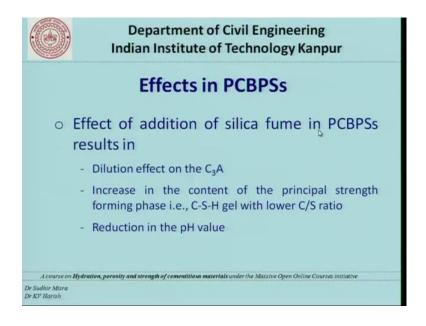
So, that is what is discussed here the effect of addition of silica fume in the mixture results in dilution effect on the C3A. So, remember that C3A stands for tricalcium aluminate and many times when you have silica fume mixture some elements of silica fume can actually react with the tricalcium aluminate.
