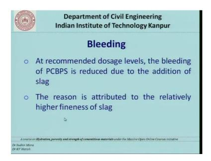
The second the important points bleeding and we find that the bleeding is reduced because of the addition of slag. And primary the reason is due to the higher fineness of slag particles. The same effect we have also seen with silica fume. So, the same thing holds good for slag also.
