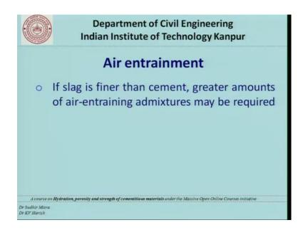
And this again depends on the fineness of slag. So, fineness of slag has a substantial effect on many properties of Portland cement based paste systems containing slag. Now
