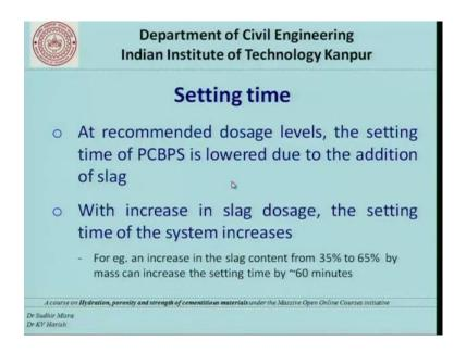
Now, coming to the setting time at recommended dosage levels the setting time of Portland cement based paste system is increased because of the addition of slag. And with increase in slag dosage beyond the recommended dosage the setting time of the system increases. So, for example, an increase in the slag content from 35 percentage to as high as 65 percentage can actually increase the setting time by 60 minutes that is very important point. When we go to setting time becomes a very important.
