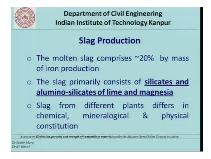
So, this again a schematic representation just to show what happens in the production of slag. Now the molten slag comprises approximately 20 percentage by mass of iron. The
