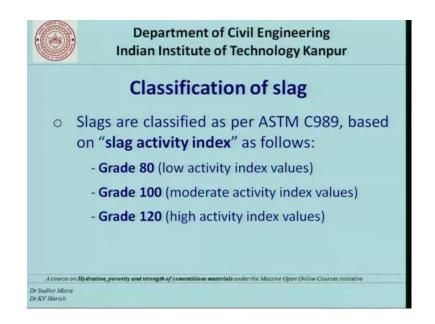
So, now coming to the classification of slag, we do not have a proper is classification for slag, but we do have some ASTM standards ASTMC 989 provides the classification for slag based on slag activity index. And based on that you have 3 different grades. Grade 80 grade 100 and grade120 and all these things are based on the strength activity index.
