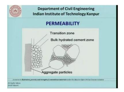
So, to explain this we will go to figure which actually shows the aggregate particle and also the cement paste which actually contains cement as well as silica fume particles.
