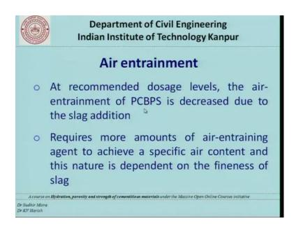
The next properties is air entrainment at recommended dosage levels the air entrainment of Portland cement based paste system decreases with addition of slag. And the this is similar to that of silica fume. And more air entraining admixtures are required to achieve the specific air content that is required.
