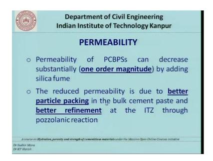
Now, next one is a permeability of Portland cement based paste system can be decreased substantially. And when we say decrease substantially it is about one order magnitude. The reduced permeability is due to better particle packing in the bulk cement paste and better refinement at the ITZ through pozzolanic reaction.
