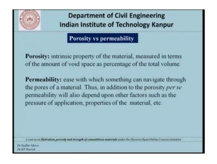
Now to review our concepts of porosity and permeability porosity is the intrinsic property of the material measured in terms of the amount of void space as a percentage of the total volume whereas, permeability is the ease with which something can navigate through the pores of that material. Thus in addition to the porosity per se what permeability would also depend upon other factors such as the pressure of application the properties of the material that is permeabiling and. so on.
