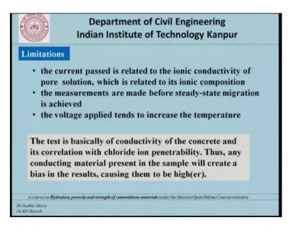
Let us understand the limitations of this test the current past is related basically to the ionic conductivity of the pore solution which is related to the ionic composition and therefore, the composition of cement and so on becomes an important parameter that could affect the results.
