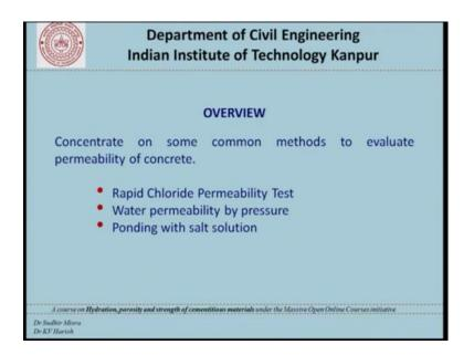
We will basically concentrate on some common methods that are available to us to evaluate the permeability of concrete and take up discussion with the rapid chloride permeability test, water permeability of concrete by pressure and ponding with salt solution. (Refer Slide Time: 00:56)
