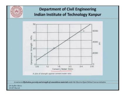
So, once we understand this I think we can move forward. This is yet another way of plotting the strength versus cement water ratio. Now very often engineers and researchers have found this to be a fairly simple way of representing the variation of strength with water cement ratio it is just the reciprocal of water cement ratio and we plot it we get more or less a straight line.
