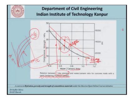
Now, here are some real numbers the compressive strength and water cement ratio if we just plot them depending on what kind of cement or what kind of concrete we have used this is just a 7 day strength with water cement ratio for concrete made with the rapid hardening Portland cement.
