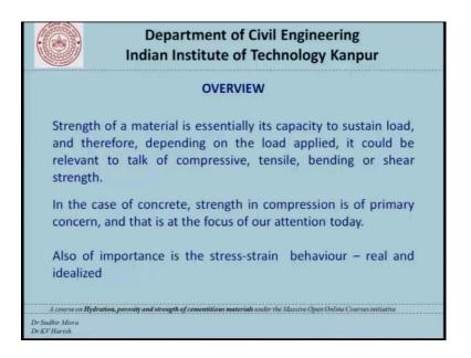
Well the strength of a material is essentially its capacity to sustain load and therefore, depending on the load applied we can talk in terms of compressive, tensile, bending or shear strength.
