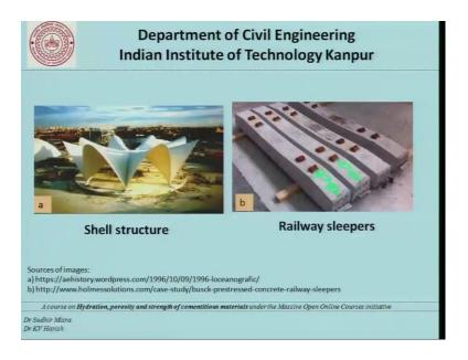
Here is a shell structure where the concrete could be very thin and made in a very difficult shape which makes the strength development, the placing of concrete, the placing of reinforcement within the concrete very difficult and that has implications on quality and therefore durability. So, we have to be extra careful when casting these kind of a special structures.
