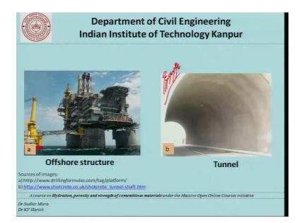
Going further this is an offshore structure, which again has the more or less. Going further this is an offshore structure which could have the same kind of a description as we have just discussed in the case of the bridge or we could make concrete tunnels. Now these tunnels have quite a different environment. On the outside of the tunnel we usually have earth or soil, and on the inside we have air. And this is largely protected from rain and so on.
