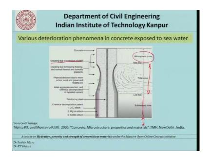
This is a model showing a concrete being exposed to sea water. We can divide the concrete into a zone where the concrete is largely exposed only to the atmospheric environment and occasional rain and so on. Then there is a tidal zone where the concrete is subjected to wetting and drying. Then there is a submerged zone and beyond that there would be a zone where the concrete is actually not submerged in water, but it is actually submerged in soil and that would be the foundations.
