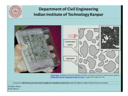
We go back to the slide a model of what concrete is, and today we will discuss how we will use this particular model of concrete having aggregate and the cement waste matrix; in the context of discussing the durability of this material when it is exposed to environmental action.
