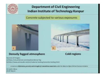
Going on there could be a concrete in dense fog, there could be a concrete bridge in very cold regions; where the discussion that I just had with you on cyclic freezing and thawing is very appropriately applicable and we need to talk of durability of such concretes as well.
