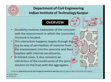
So, now durability involves interaction of the concrete with the environment in which the concrete structure is located. Basically we have this concrete which is interacting with the environment outside. And we must understand that the durability of this material is very close to be related to the environment in which it is located. So, that is what is the first of our discussion today.
