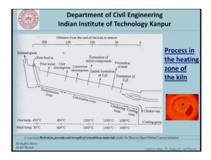
So, what you see in the figure is the kiln which is inclined at some angle and at one end of the kiln you will see the fire that is provided for which you need some fuels which is already discussed in the previous slide and at the other end the raw materials are fed.
