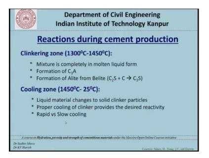
In the clinkering zone, 1,300 degree Celsius to 1,450 degree Celsius, the mixture is completely in molten liquid formation of C3A takes place formation of Alite from Belite that is C 2 S reacts with C to give C3S remember that C does not refer to carbon C refers to calcium oxide.
