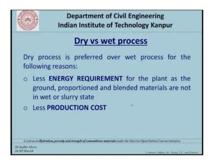
So, dry process is preferred over wet process for the following reasons in dry process the energy that is required is much less for the plant as the ground proportion and blended materials are not in the wet or slurry state in addition in the dry process the production cost is very low.
