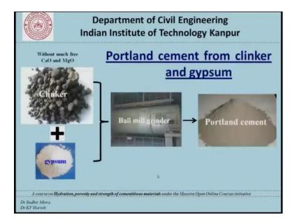
So, once the raw materials comes out after the burning process it is called as clinker and we need to make sure that it does not contain too much of free calcium oxide or magnesium oxide and then it is added to gypsum and both are fed in ball mill grinders and once it is ground well then you get the material called Portland cement which will be in fine particle form and they are packed in bags and distributed.
