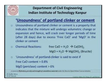
Unsoundness of Portland cement is a property that indicates that the mixture will undergo volumetric change or expansion or cracking over longer periods of time usually after 28 days due to excess amounts of either free calcium oxide which is not properly burnt or magnesium oxide that is present in the clinker or due to both free calcium oxide and magnesium oxide.
