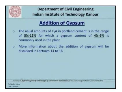
The usual amounts of tri-calcium aluminate in Portland cement is in the range of 5 to 12 percent for which the gypsum content is in the range of 4 to 6 percent and hence this quantity is used commonly in the plant more information about the addition of gypsum will be discussed in lectures 14 to 16.
