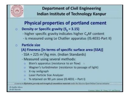
Physical properties of Portland cement; so, the main important properties of Portland cement alone are discussed first one is density or specific gravity the specific gravity of Portland cement typically is 3.15 that value is very important higher specific gravity usually indicates that the quantity of tetra calcium alumino ferrite is higher in Portland cement the density or specific gravity is measured using Le chattier Apparatus and the procedure for this is given in IS 4031; part 2.
