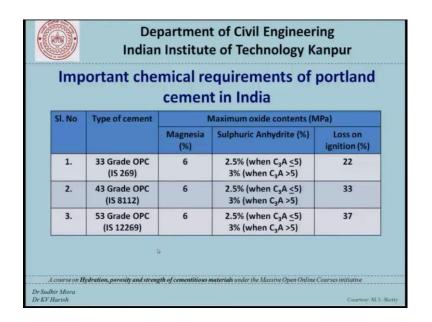
The chemical requirements of Portland cement in India are shown in this table for the 33 grade, 43 grade and 53 grade, the magnesia content should not exceed 6 percent, for all the 3 types of cement sulphuric anhydrite content should not exceed 2.5 percent when Tri-calcium aluminate content is lower than or equal to 5 percent and it should not exceed 3 percent when Tri-calcium aluminate content is greater than 5 percent and the
