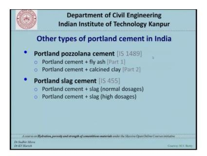
In addition to the different grades of cement available we also have other types of Portland cement namely Portland pozzolona cement specified in IS 1489 and in this, there are again 2 types of cement, 1 is Portland cement with fly ash and Portland cement with calcined clay they are given in port part 1 and part 2 of IS 1489.
