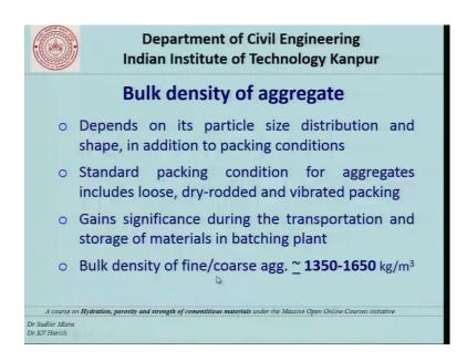
Bulk density of aggregate depends on it is particles size distribution shape in addition to packing conditions. Standard packing conditions for aggregates include loose packing, dry rodded packing and vibrated packing; bulk density of aggregate gains significance during the transportation and storage of materials in batching plant. And usually the bulk density values for fine or coarse aggregate is in the range of 1350 to 1650 kg per meter cube.
