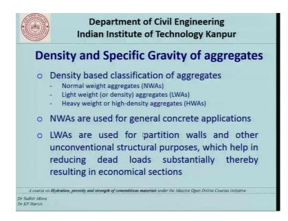
Aggregates may be classified based on density as normal weight aggregates or normal density aggregates indicated as NWA, light weight or light density aggregates indicated as LWA, heavy weight or high density aggregates indicated as HWA. Normal weight aggregates are used for general concrete applications, light weight aggregates are used for partition walls and other unconventional structural purposes which help in reducing dead loads substantially thereby resulting in economical sections.
