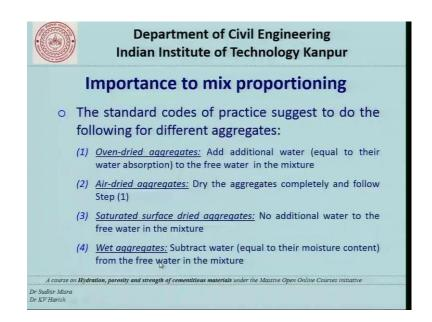
The standard codes of practice suggest to do the following for different aggregates. If you have the over dried aggregate, then add additional water that is equal to their water absorption to the free water in the mixture. If you have a air dried aggregate dry the aggregates completely and follow step one.
