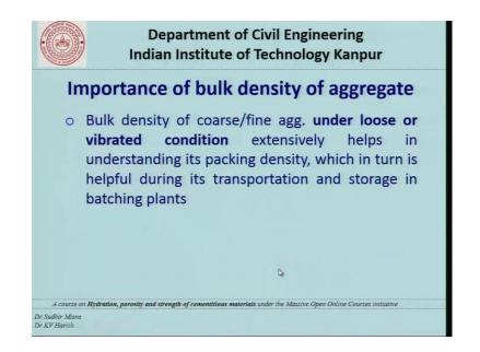
The third importance is that bulk density of coarse of aggregates under in loose or vibrated condition extensively helps in understanding it is packing density which in turn is helpful during it is transportation and storage in batching plants.
