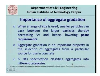
Now, some important information about aggregate gradation when a range of size is used smaller particles can have packed between the larger particles, thereby decreasing Vv which is volume of voids and hence lowering paste requirements. Aggregate gradation is an important property in the selection of aggregates from particular source for use in concrete IS 383 specification classifies aggregates into different categories.
