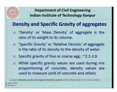
The next is important property is density and specific gravity of aggregates. Density also referred as mass density, is a ratio of it is weight to it is volume. Specific gravity or relative density of aggregate is a ratio of it is density to the density of water. Specific gravity of fine or coarse aggregate is usually in the range of 2.2 to 2.8. While specific gravity values are used during mix proportioning of concrete density values are used to measure yield of concrete and others.
