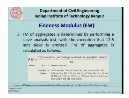
Fineness modulus of aggregates is determined by performing a sieve analysis test with the exception that 12.5 mm sieve is omitted. Fineness modulus of aggregates is calculated by using the following formula. Fineness modulus equal to summation of cumulative percentage retained on specified sieves divided by 100. And the specified word is very important because only certain sieve source specified.
