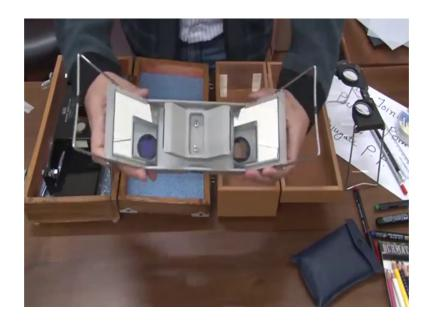
This is having mirror on both its legs right and left so, this will give the reflection of the photographs and these reflections will move to this mirror ok. So, this mirror are located on the is (Refer Time: 22:07) angular plates so, now, the this will finally, reflect your image on these two lenses, through which you can generate your 3 D vision by putting your photographs below this like this ok.
