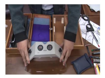
Here another kind of stereoscope you can see this is this stereoscope means from Sokkia company made in Japan, this is a simple kind of stereoscope.
