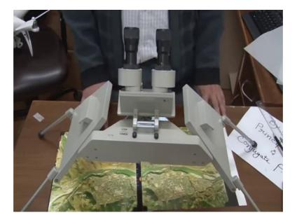
This is the binocular used to set for magnifying view of the photographs and here this is the mirror stereoscope. So, I am showing you with the front side of it so, that you can see it easily.
