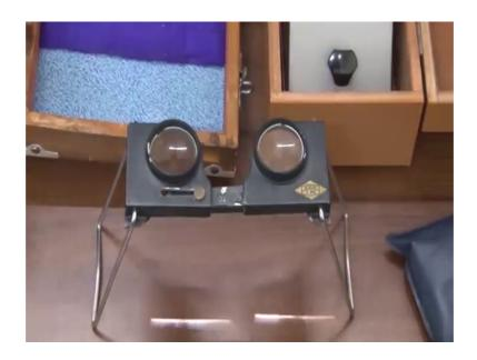
So, as you can see right this is a pockets stereoscope, this is a portable kind of thing which you can carry with you in the field also if you are taking some out going to carry some topographic survey with you with taking aerial photographs. So, this is a portable set of stereoscope so, this is called the pocket or lens stereoscope.
