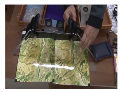
So, this is other medium size of stereo scope is also called mirror stereoscope because it is having set of mirror on both the sides. As you can see here these are the plates on both its legs and here also this will give you direct vision not through a second mirror.
