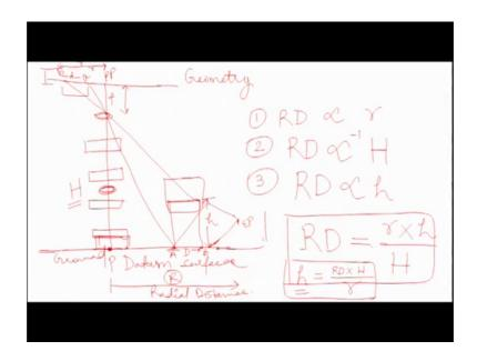
So, now after having an understanding of relief displacement, let us try to understand it in a very simple geometry. So, that you do not have any confusion, while doing your practical's. So, suppose this is your ground ok, let us draw this ground lower. So, this is your ground which is taken by the lens mounted on a camera, this is the altitude of your camera, altitude of your flying height you can say, this is your datum surface simply data and suppose this is a building over this plane.
