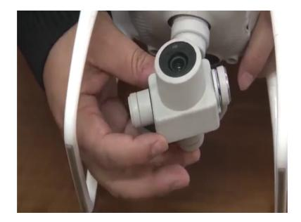
So, this is a model this model is known as phantom pro and here the lens is placed ok. So, this is a lens having a high magnification ok, a high power which can look over the ground and capture ground from a greater height also.
