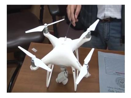
So now let us have some other kind of photograph. So, as you can see here, this is an UAV means unmanned aerial vehicle. So, this can take photographs of the ground, in the same manner a satellite or an aircraft takes ok. So, this with the help of this UAV you can also take photographs in a sequence, along a line of flight the overlapping photographs these are the wings ok.
