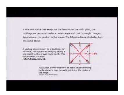
One can notice that except for the features on the nadir point, or the principal point. As you can see here, in this case of aerial photograph this will be the fidition marks, on these photographs on all the four edges, now on the midpoint of the edges. So, this will be the line joining the fidition marks will be your principal point.
