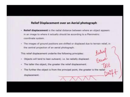
So, what is a relief displacement in terminology, it is the radial distance between where an object appears, in an image to where it actually should be according to a Planimetric coordinate system ok.
