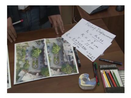
So, this will go with this capital R into H divided by r. So, here this H represents the height of the object or the height of the building, capital R represents a relief displacement H represents height of a flying altitude, and a small r represents the radial distance from the principal centre, and what is the radial distance from the principal centre?
