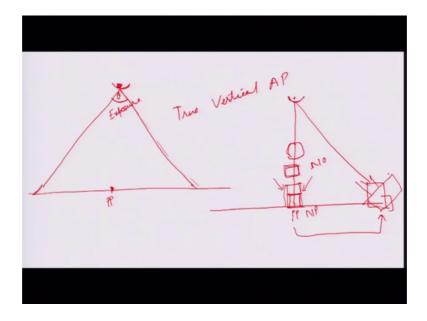
So, as we know that; when we take a photograph with a single camera it will cover an area with central projection ok. Central projection; means there is the rays will be projected from a center, that is your camera aperture and it will cover an area like this and this will be your exposure and this will be your coverage angle ok.
