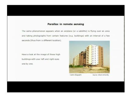
Here an example of a high building from Cairo, Egypt. So, this building; the same building was taken by Ikonos satellite from 2 different positions of its sensors ok. So, the same phenomena appears when an airplane or a satellite is flying over an area and taking photographs from certain features or buildings with an interval of a few seconds does from a different location.
