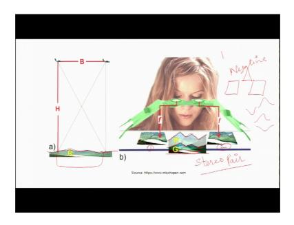
Suppose this is a terrain and undulating terrain of course, so, but how you can see the relief of this terrain? When you see the 2 different photographs of the same terrain taken by a camera onboard an aircraft; So, here these 2 photographs are the stereo pair; so, in this way you will have depth perception what is the meaning of depth perception?
