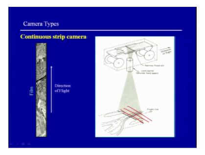
Then you are having Continuous strip photography, which has been shown here this is your camera mounted and you have the direction of the flight, which has been shown here also, and it will keep collecting the picture like this. So, this is one strip then you will have another one here, then you will have 3rd one here, then you have 4th one here and this will have an overlap, if you want to have the these stereo images.
