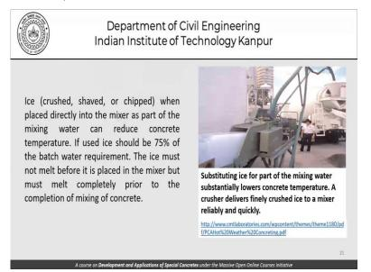
Here is a plant showing ice being substituted as a part of mixing water which substantially lowers the concrete temperature. And a crusher delivers finely crushed ice to a mixer reliably and quickly. So, one has to be very careful when using ice. There are different ways of doing it crushed shaved or chipped dice is what is used and that when placed directly into the mixer as part of the mixing water can reduce the concrete temperature.
