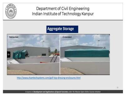
Now this is a picture which I have taken from the previous discussion. It is a retracted and extended aggregate storage system and that is something which we can use in hot weather as well as in cold weather conditions because at the end of it what we need is to control or kind of engineer the temperature of aggregates. If you want to heat it, we want to cool it, it is better to protect it from the ambient or the outside air temperatures and air effects.
