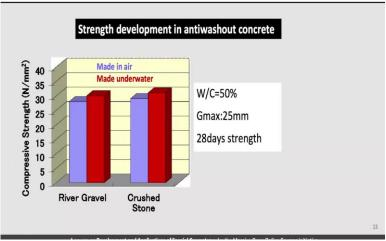
This here is a representation of the strength development in anti-washout concrete and you can see here that the concrete is very much a normal concrete water cement ratio 50%, 25 mm of maximum size aggregate and we are talking of 28 days strength as usual. If you are using river gravel or crust stone made in air or made in water or made under water the strengths are not drastically different, they are just marginally different.
