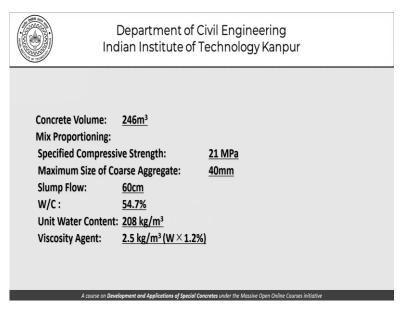
This is yet another example that 146 cubic meters of concrete has been used with 21 MPa the required strength 40 mm aggregate 60 centimetres slump flow 54.7% of water cement ratio and the water content being 208 and here we are talking of a viscosity agent at 1.2% of water which turns out to be about 2.5 kgs per cubic meter. So, the amount of viscosity agent is very small but its effect is very, very significant. As far as the properties concrete are concerned.
