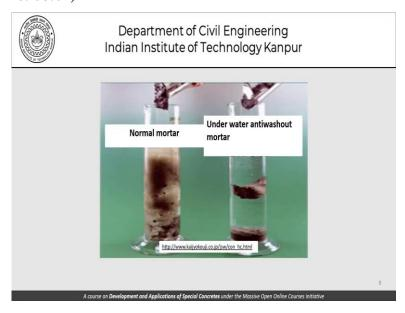
Now this picture showing normal mortar and underwater anti-washout mortar being placed in a measuring cylinder of water shows the picture as to how the underwater concrete or the anti-washout underwater concrete is so different from normal concrete. Normal concrete would involve this kind of segregation or a washout of cement particles or even fine sand particles from the mortar once it is dropped in water.
