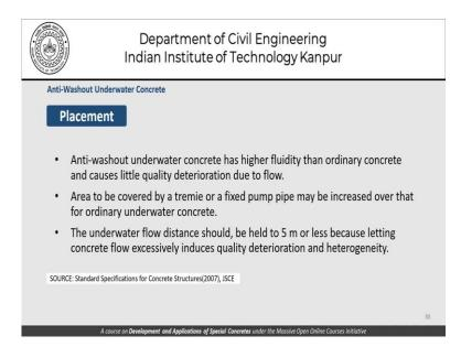
The anti-washout concrete has higher fluidity than ordinary concrete and causes little or no deterioration as far as flow is concerned. Ideally placed anti-washout concrete has higher fluidity than ordinary concrete and properly placed. There is no cause for any deterioration in the quality due to flow. Area to be covered by a tremie or a fixed pump pipe may be increased compared to an ordinary underwater concrete.
