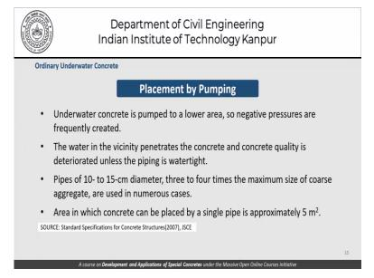
When we are trying to place concrete by pumping. Underwater concrete is pumped to a lower area negative pressures are frequently created and the water in the vicinity penetrates the concrete. In the concrete quality deteriorates unless the piping is watertight. So, pipes of 10-50 centimetres diameter which is three to four times the maximum size of the coarse aggregate are used in numerous cases.
