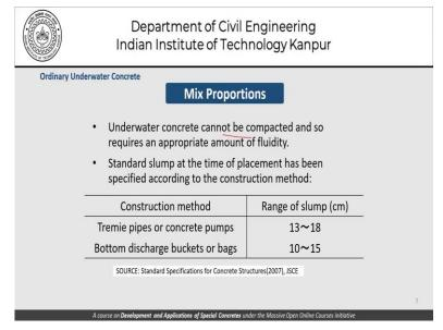
So as far as the ordinary underwater concrete is concerned the proportions of this concrete have to be determined keeping in mind the fact that underwater concrete cannot be compacted. And so, it requires an appropriate amount of fluidity to begin with standard slump values at the time of placement have been specified according to the construction methods. For example, the JSC tells us that if we are using tremie pipes or concrete pumps.
