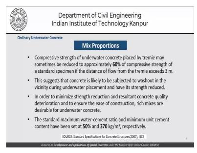
Compressive strength of underwater concrete placed by tremie may sometimes be reduced to approximately 60% of the compressive strength of a standard specimen if the distance of flow from the tremie exceeds 3 meters. An appropriate account of that has to be made that suggests that concrete is likely to be subjected to wash out in the vicinity during underwater placement and have its strength reduced.
