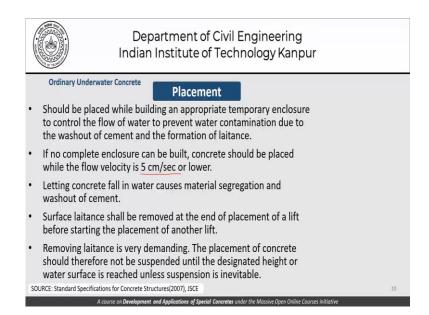
As far as placement is concerned when we are using ordinary underwater concrete. The concrete should be placed while building an appropriate temporary enclosure to control the flow of water and to prevent water contamination due to the washout of cement and formation of latent. If no complete enclosure is built or if no complete enclosure can be built concrete should be placed at least by ensuring that the flow velocity has been reduced to 5 centimetres per second or lower.
