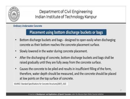
When we are using bucket discharges or bags as a placement method they are designed to open easily when discharging the concrete as the bottom reaches the concrete placement surface. They are slowly lowered into the water during concrete placement and discharging the concrete the bottom discharge bags or buckets are gradually raised until they are fully away from the concrete surface.
