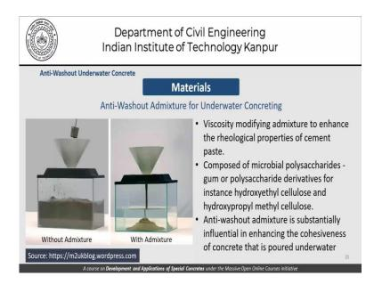
So, this picture here is just a representation of what we saw last time also that without the admixture we have this kind of a slightly murky or a muddy picture as far as reinforcement is concerned. Whereas here with the admixture that is the viscosity agents the viscosity modifying admixtures that we are calling them we can see that the mortar is being placed very cleanly and is settling within the water tank.
