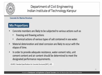
Coming to the mixed proportions for concrete and marine structures the concrete members are likely to be subjected to various actions as freezing and thawing depending on the temperatures involved. Chemical action of various types of salts contained in sea water. And what we are encountering is two situations the material deterioration of concrete and the steel corrosion these two things are likely to happen over a long period of time.
