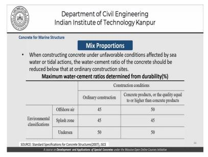
When constructing concrete under unfavourable conditions affected by sea water or tidal action which is typical in the case of marine structures. The water cement ratio of the concrete should be reduced and in fact this table tells us the maximum water cement ratio values determined from durability considerations depending upon the environmental classification. Of course, this environment classification is different from the environment classification given in IS456.
