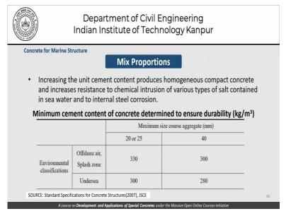
Apart from the water cement ratio there are requirements for the unit cement content and this table here talks about the minimum cement content of concrete determined to ensure
