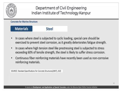
As far as steel is concerned in cases where steel is subjected to cyclic loading special care needs to be taken to ensure prevention of corrosion as it could greatly reduce the fatigue strength. In cases where high tension steel like pre-stressing steel is subjected to stress exceeding 60 of its tensile strength the steel is likely to suffer stress corrosion. As well and appropriate counter measures need to be taken in that case.
