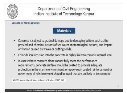
And concrete in marine structures is subject to gradual damage due to damaging action such as physical or chemical actions of sea water metallurgical actions and impact or friction caused by waves or drifting solids in the sea. Chloride ion penetration into concrete is highly likely to corrode the internal steel that we have if it is a reinforced concrete structure. And in cases where concrete alone cannot meet the performance requirements.
