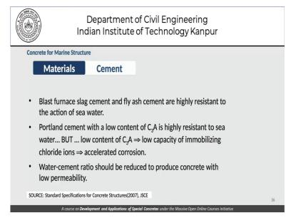
The blast furnace slag cement and fly ash cements are highly resistant to the action of seawater, Portland cement with a lower C 3 A content is highly resistance to sea water. But with the low C 3 A it has a lower capacity for immobilizing the chloride ions and therefore it can have some implications as far as corrosion is concerned. Water cement ratio should be reduced to produce a concrete with a low permeability.
