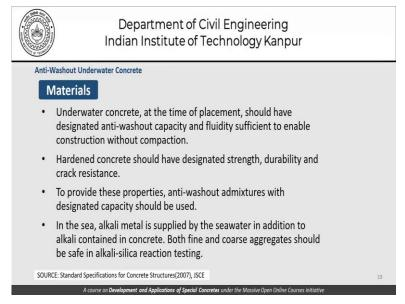
Now coming to our discussion on the special anti-washout underwater concrete that's what we saw in our last discussion. As far as the materials are concerned in underwater concrete at the time of placement should be designated to have the right kind of anti-washout capacity and fluidity sufficient to enable the construction without compaction. Hardened concrete should have the designated strength durability and crack resistance and provide these parameters.
