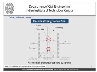
So, we may need to use flange joints as shown here because those pipes come in certain lengths and make sure that this end always remains in the concrete it has been placed. And the diameter here over which we can use a single tremie is also given to you the 30 square meter guideline. So, these are some of the things that you can take as guidelines when you are using underwater concrete ordinary underwater concrete using a tremie and doing underwater construction.
