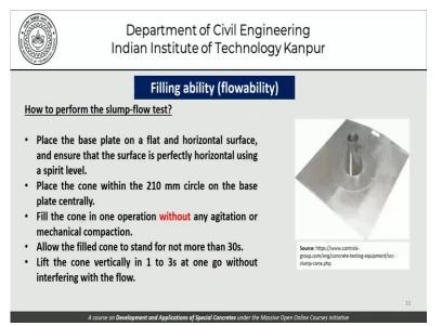
As far as the procedure to perform the slump flow test is concerned place the base plate on a flat and horizontal surface and ensure that the surface is perfectly horizontal using a spirit level. Place the cone within 210 millimeter circle range of the base plate centrally. So we have a circle which is already marked here and that a circle measures 210 because the slump cone itself is 200. Fill the cone in one operation without any agitation or mechanical compaction.
