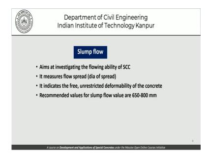
So as far as the slump flow is concerned that aims to investigate the flowing ability of the self-compacting concrete it measures the spread which is in terms of the diameter of the spread. Remember that the bottom of the slump cone is 200 mm that is the bottom diameter of the slump cone. So how much it spreads from there is really the slump flow that we are talking about as we should see also.
