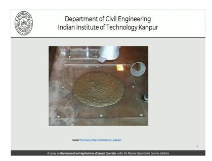
This picture here shows the spread that has been achieved after the slump cone has been removed and this diameter is what we are talking about as the slum flow. As we shall see just now the procedures call for measurement of two diameters and try to take the average provided it is not highly skewed and so on and so forth. A corollary to the slump flow is the flow time called the T 500 test.
