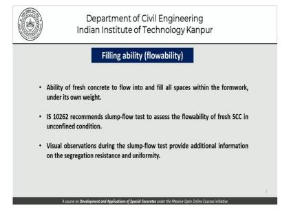
Now coming to the; first one which is the filling ability which is flow ability, the ability of fresh concrete to flow into and fill all spaces within the form work under its own weight this is what is the definition or this is what we can define fill ability or flow ability as. IS 10262 recommends the slump flow test to assess the flowability of fresh self-compacting concrete in unconfined condition.
