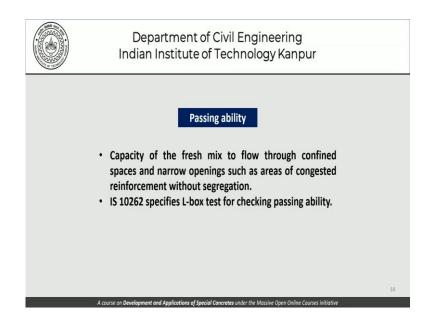
Now remember that the slump flow test is unrestricted flow of concrete that measures unrestricted flow of concrete without any obstructions. Compared to that the passing ability test is the capacity of the fresh concrete to flow through confined spaces and narrow openings such as the areas of congested reinforcement without segregation. Go back and try to look at the picture of congested reinforcement and that should always be at the back of your mind.
