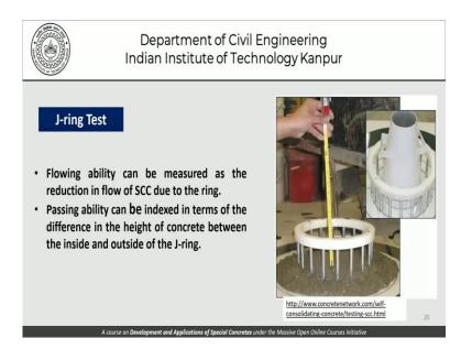
Now the flowing ability can be measured as the reduction in the flow of the concrete due to the ring and the passing ability can be indexed in terms of the difference in the height of concrete between the inside and the outside of the J-ring. So we can measure the height of concrete inside the ring and outside the ring and I am leaving it to you to read a little bit more about where exactly these measurements have to be carried out as far as the inside of concrete is concerned.
