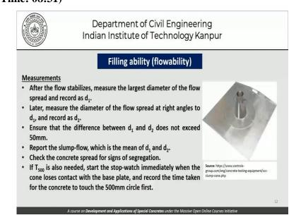
As far as the measurements are concerned after the flow stabilizes measure the largest diameters of the flow spread and record it as  $d_1$  later measure the diameter of the flow spread at right angles to  $d_1$  and record it as  $d_2$ . Ensure that the difference between  $d_1$  and  $d_2$  does not exceed 50 mm. And report the slump flow which is the mean of  $d_1$  and  $d_2$  which means it is  $(d_1 + d_2)/2$ . Check the concrete spread for the signs of segregation.
