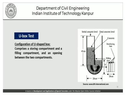
Moving forward we have the U-box test. So the configuration of the U-box test basically is it comprises a storing compartment and a filling compartment and an opening between these two compartments. So this here is my storing compartment and this here is my filling compartment. The concrete is stored here and allowed to move through this gate into this filling chamber. The gate here is shown in this picture here and we can see that there is some kind of simulated reinforcing bars also.
