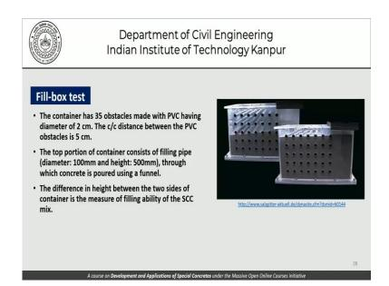
So moving forward we come to the last test that I have in my plan today that is the fill box test and this container has 35 obstacles. These 35 obstacles if you want to count them it is 1, 2, 3, 4, 5 and 6, 7 and arranged in 5 layers and we put the concrete here all over the place and then we try to see how it negotiates the space between simulated reinforcing parts. This test actually simulates the flow of concrete not through one layer only.
